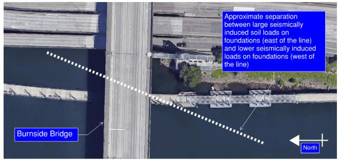
Figure 2: Plan at Existing Bridge Showing Approximate Location of Liquifiable Soils
