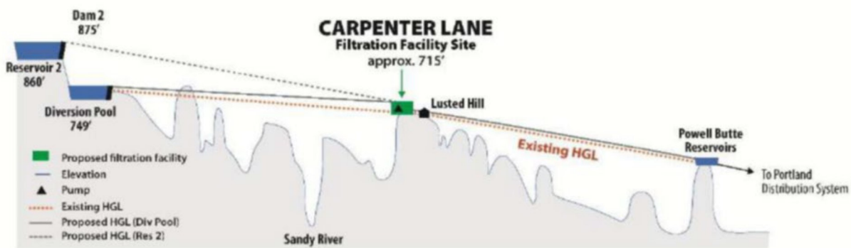
Figure 21. Diagram of gravity flow from Bull Run to Portland
