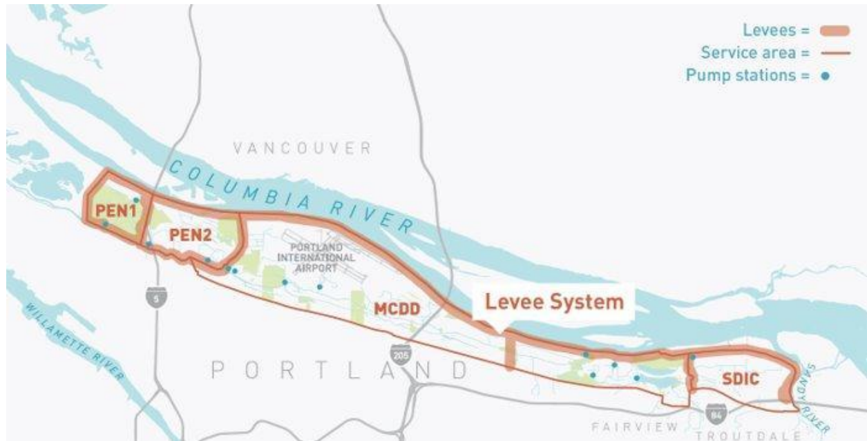
Figure 50 - Map showing the boundaries of the four current Columbia Corridor Levee Districts, along with the locations of the levees themselves and pump stations. Map from the Multnomah County Drainage District.
