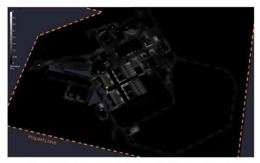
Figure 2. Simulation of Facility lighting with all fixtures dimmed.
