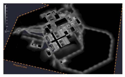
Figure 1. Simulation of Facility lighting with all fixtures at full brightness.
