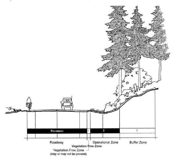
Figure 2. Right-of-way maintenance zones.
