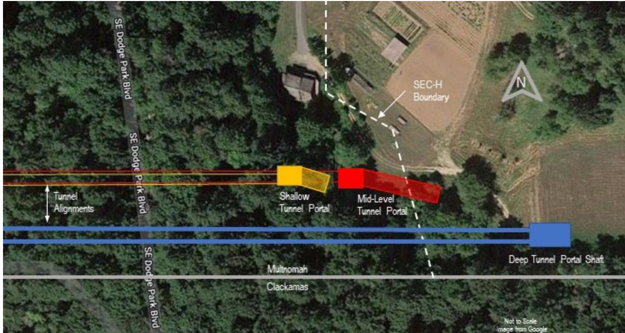
Figure 6. Tunnel Portal Alternatives Relative to SEC Zone
