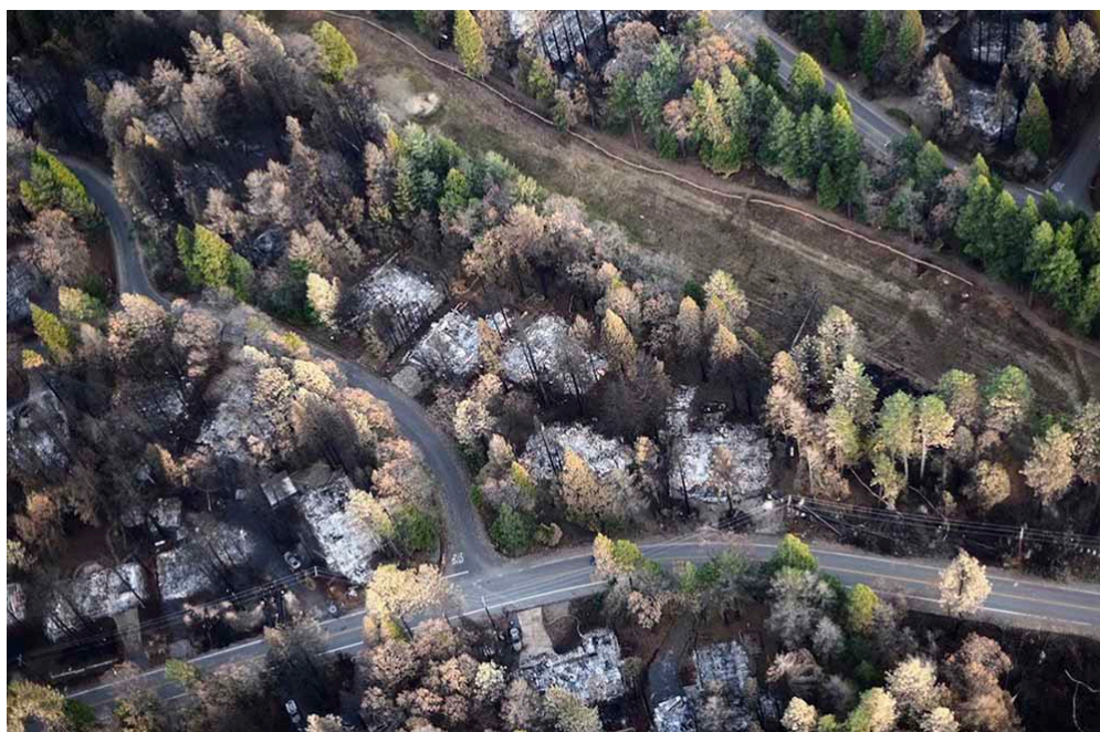
Figure 41 - Aerial photo of damage from the 2018 Camp Fire in California. Structures have burned to the ground even as much of the adjacent vegetation has survived the fire. In some locations, trees suffered more damage from being in proximity to burning homes than from the main line of wildfire. Photo – Owen Bettis, Deer Creek Resources
