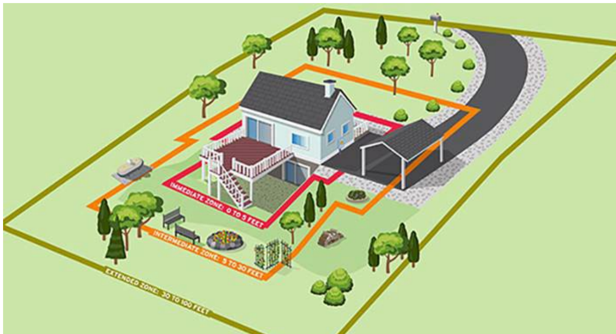
Figure 42 - Diagram showing the home ignition zone. National Fire Protection Association
