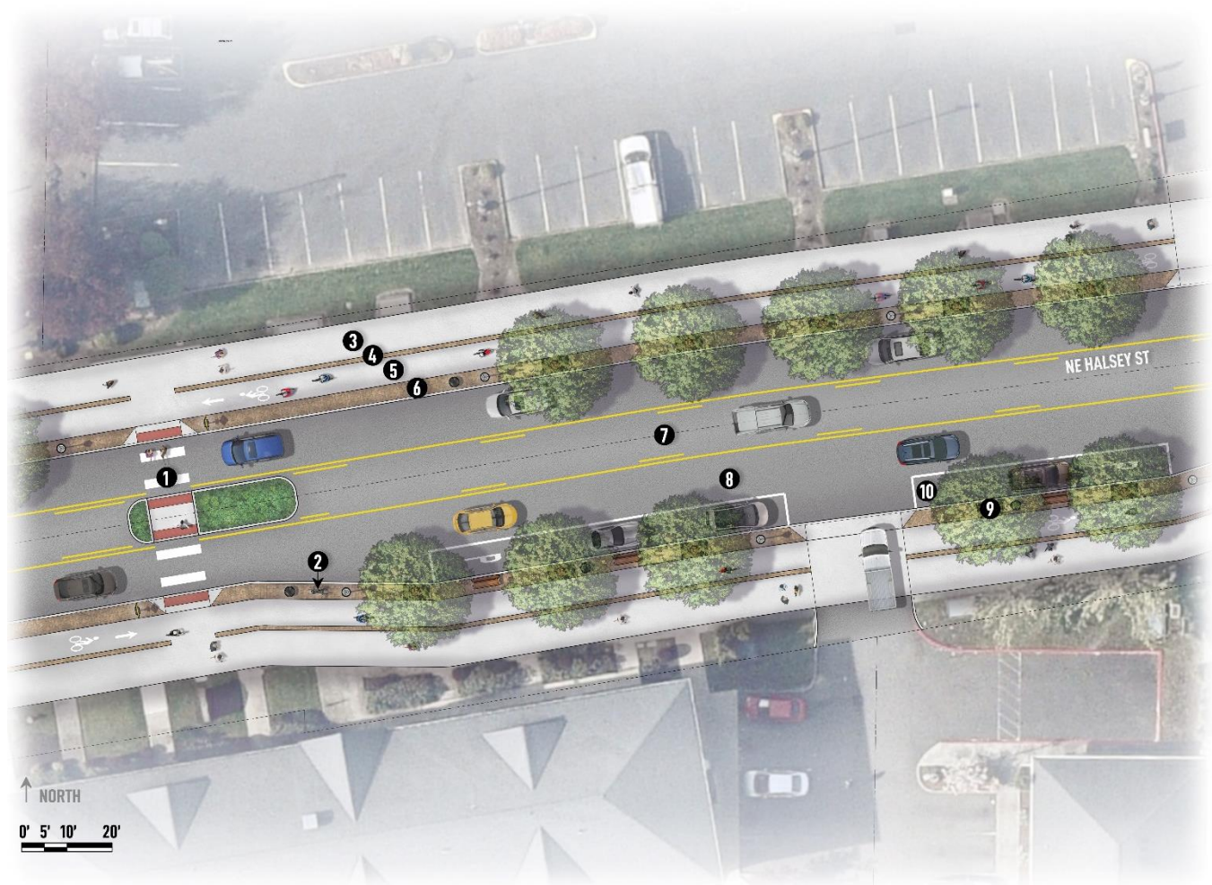
Figure 21: Typical Corridor On-Street Parking Layout (West of NE Halsey St and NE 238 th Drive)
