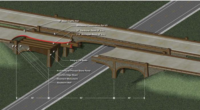
Pedestrian underpass and abutment wall/slope detail
