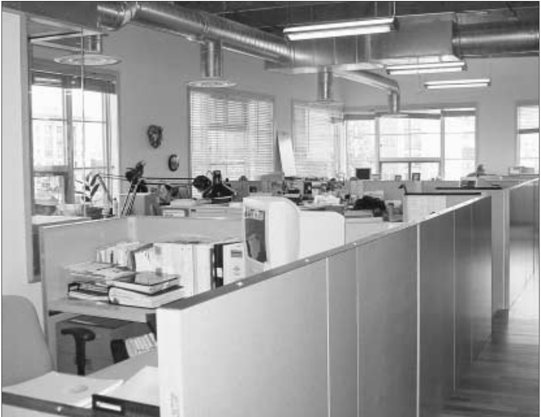
Workstations built from recycled doors.
