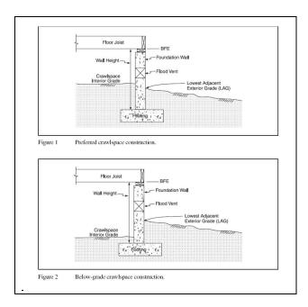
(a) The interior grade of a crawlspace below the base flood elevation shall not be more than two feet below the lowest adjacent exterior grade.
