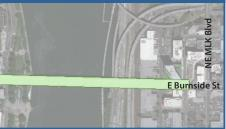
A new fixed bridge with a maximum clearance of 97 feet, at about the same location as the current bridge. It doesn't open, but is tall enough to allow ships to pass without halting traffic. The west landing touches down about 3 blocks further west than the current bridge, near NW 5th Avenue.
