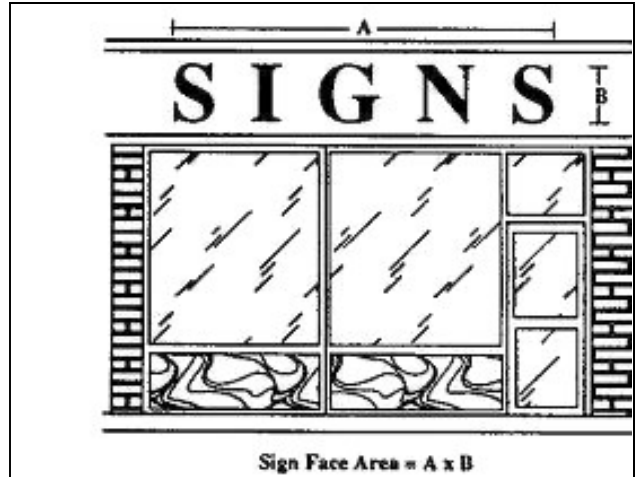
Figure 4 – Sign Face Measurements
