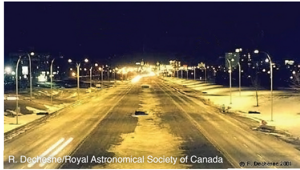
R. Dechesne/Royal Astronomical Society of Canada Notice the glare of the old drop lens fixtures in the background compared to the new flat-lens fixtures in foreground, Calgary, Alberta, Canada.
