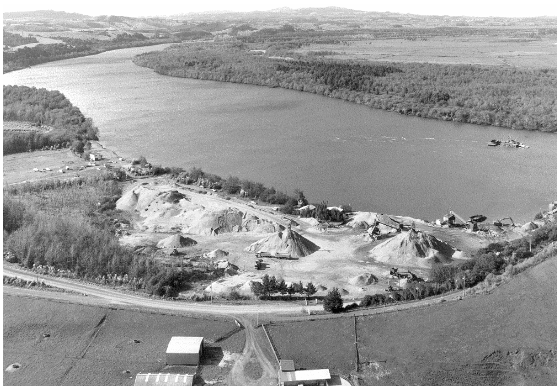
Figure 1: Extraction processes and material stockpiles are common sources of wind-blown dust
