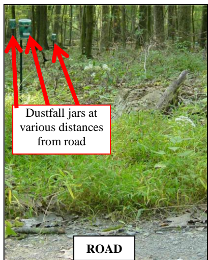
Figure 9. Distance experiment; dust fall jars on buffer site 2-3.
