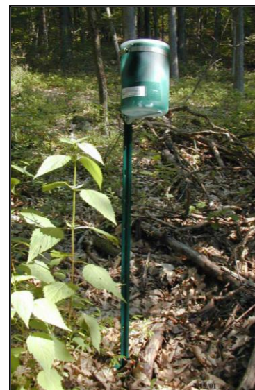
Figure 7. Typical dust fall jar placement.
