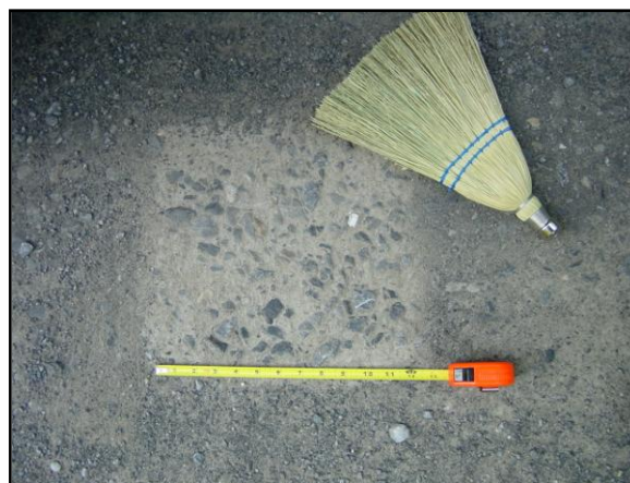
Figure 11. Example of 1 foot square used to obtain a sweep sample
