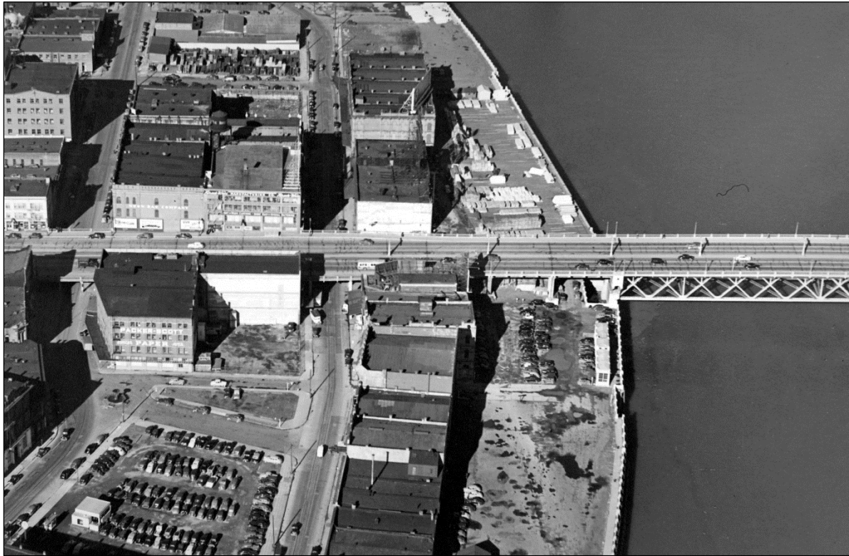
Figure 5-41. Aerial view of the Harbor Wall area around the western end of the Burnside Bridge in 1935. Note the Harbor Wall did not connect with the bridge pier.
