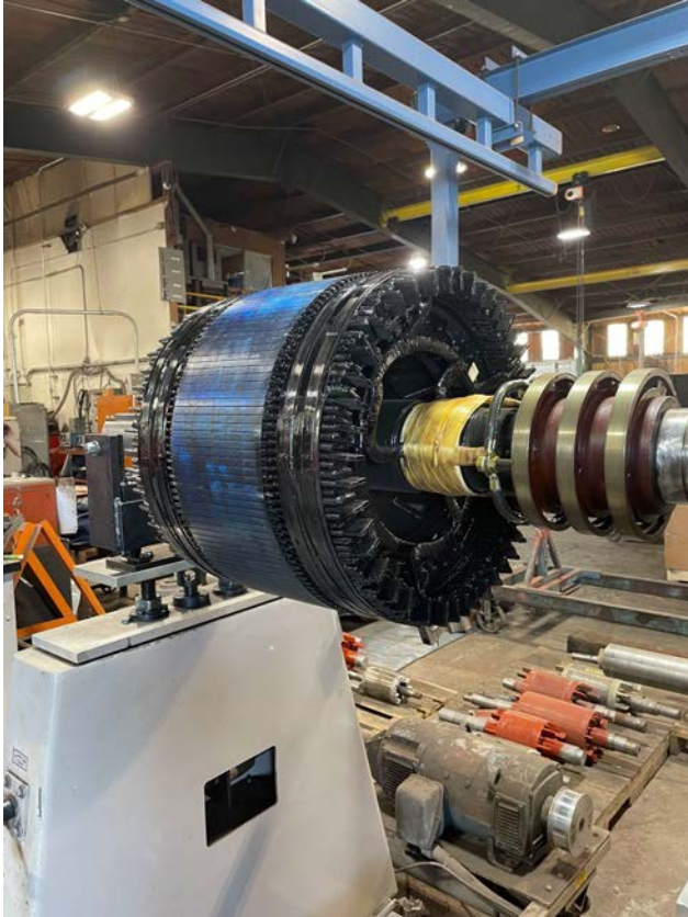
Refurbishing of the existing motor
