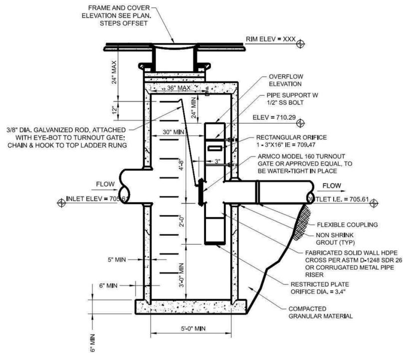
**A** Flow Control Maintenance Hole - Pond A
