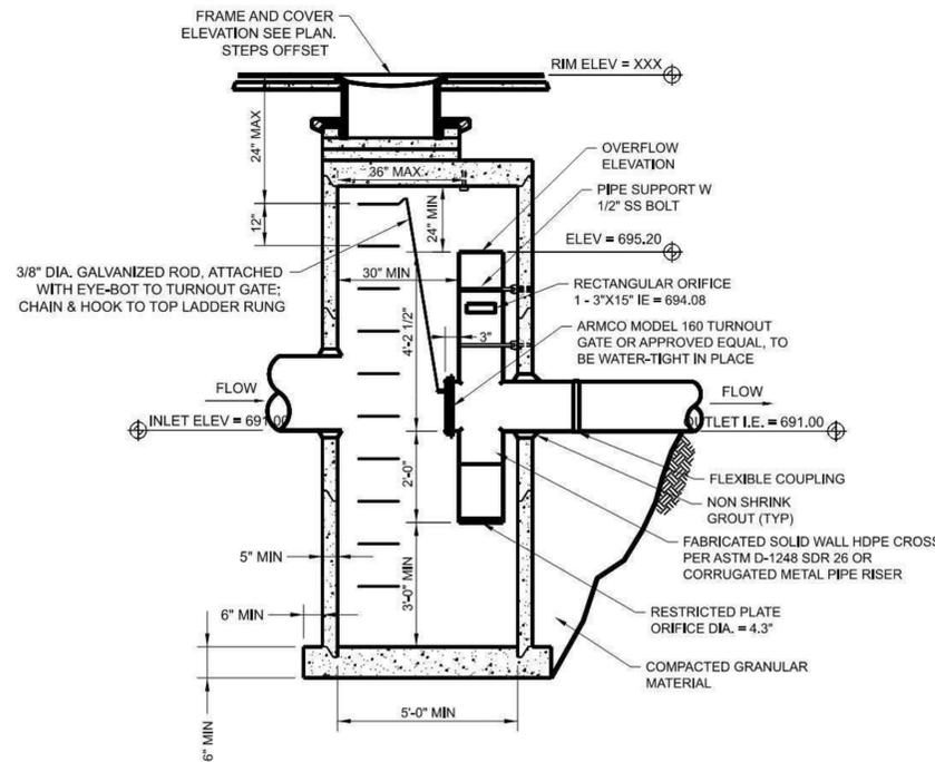
**D** Flow Control Maintenance Hole - Pond D
