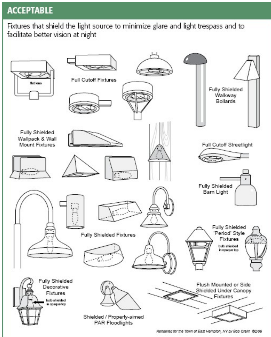
Figure 13 Acceptable Light Fixtures
