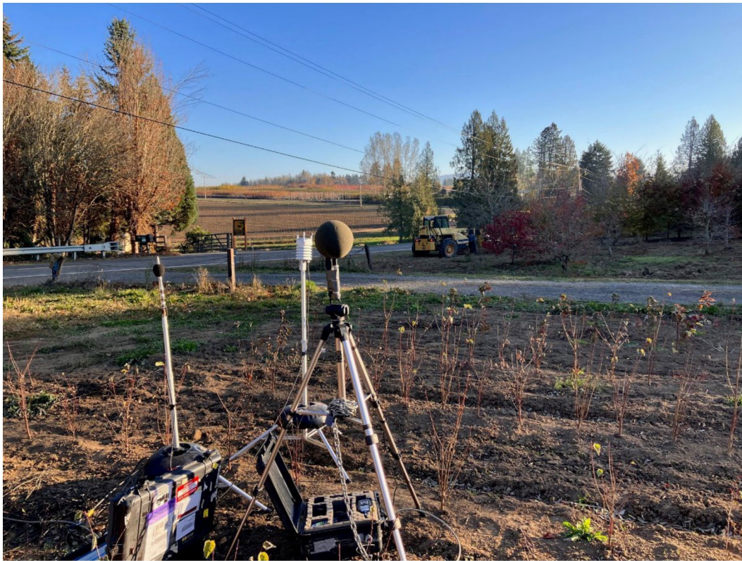
Figure 2-3. Noise Monitoring Equipment Looking Northeast (SE Lusted Road in Background)
