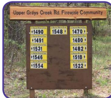
**Address:** The home address should be readily visible from the street. The address sign should be made of reflective, noncombustible material with characters at least 4 inches high. With multiple homes, use reflective directional arrows to ensure that responders can quickly find your home.
