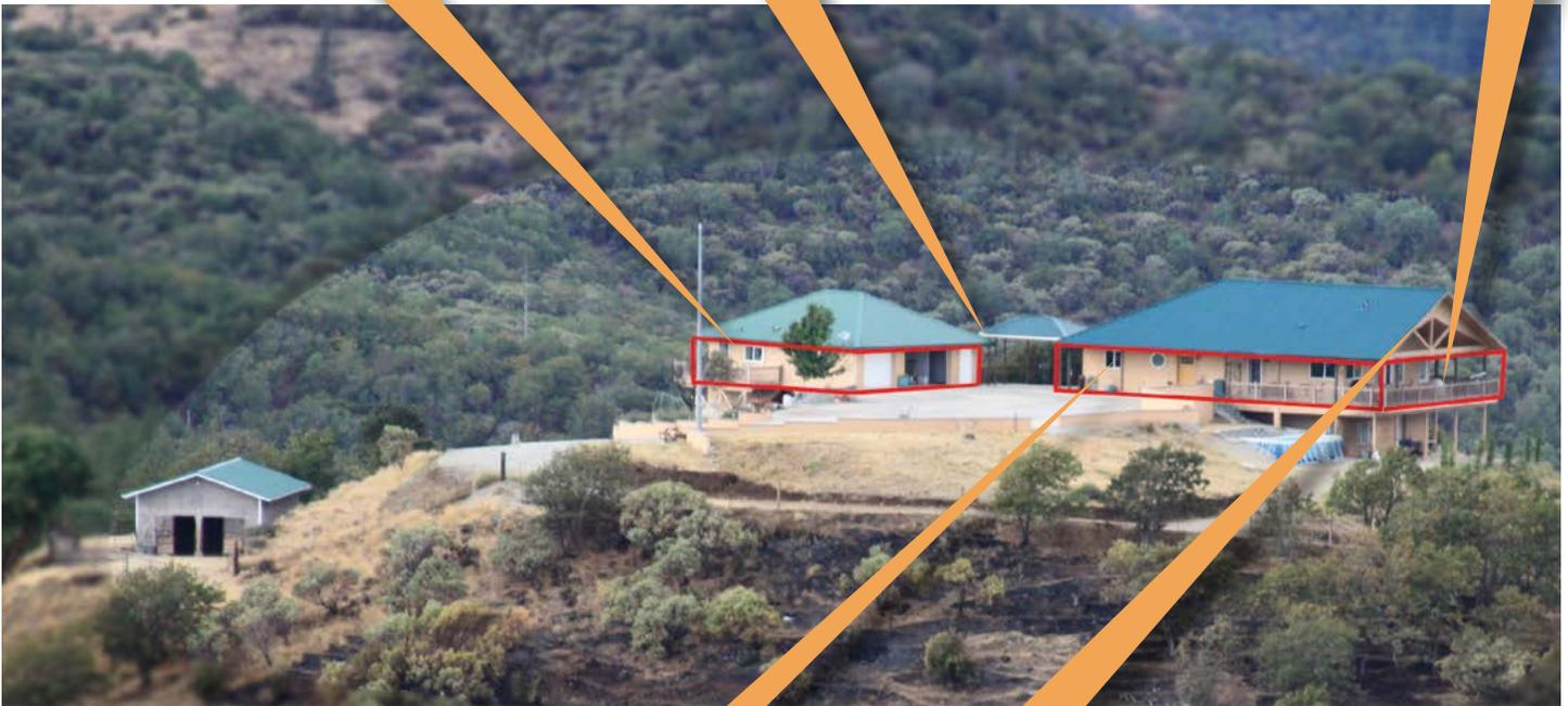
Windows are one of the weakest parts of a home in a fire, usually breaking before the house ignites. Double-paned windows with tempered glass are less likely to break. Closable, solid exterior shutters can provide extra window protection.
