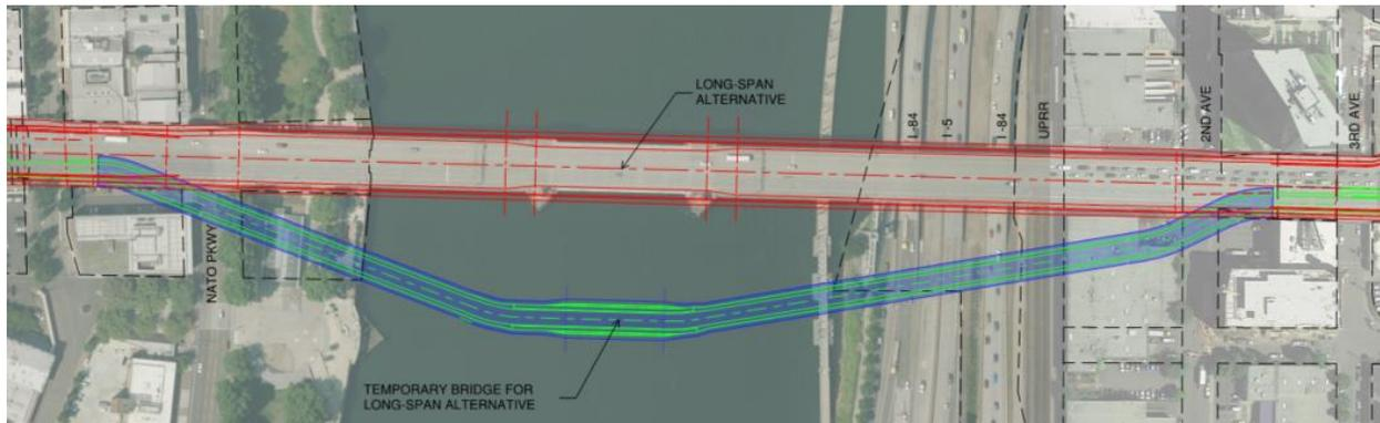
The temporary bridge could consist of fixed spans along the east and west approach, and a movable lift span within the river navigation channel. This would allow for demolition of the majority of the existing bridge spans and construction of the replacement spans to occur. However, because the temporary bridge cannot tie in past the existing bridge tie in without large ROW impacts, a portion of both the east and west approach spans would need to be constructed in stages.
