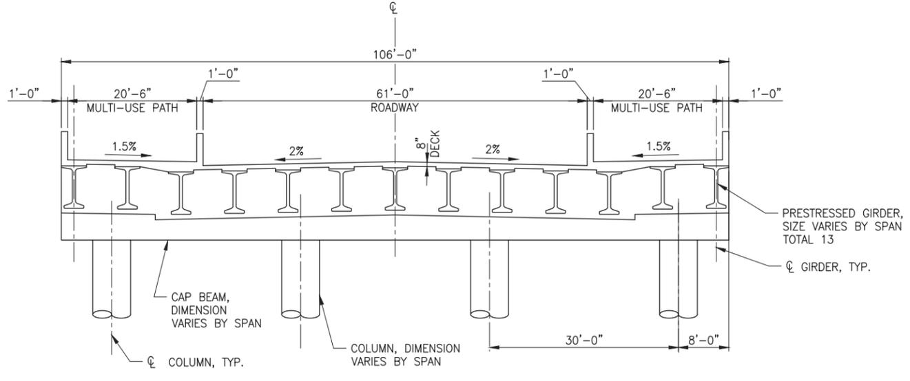
**FULL WIDTH TYPICAL SECTION - PRESTRESSED CONCRETE GIRDER**
