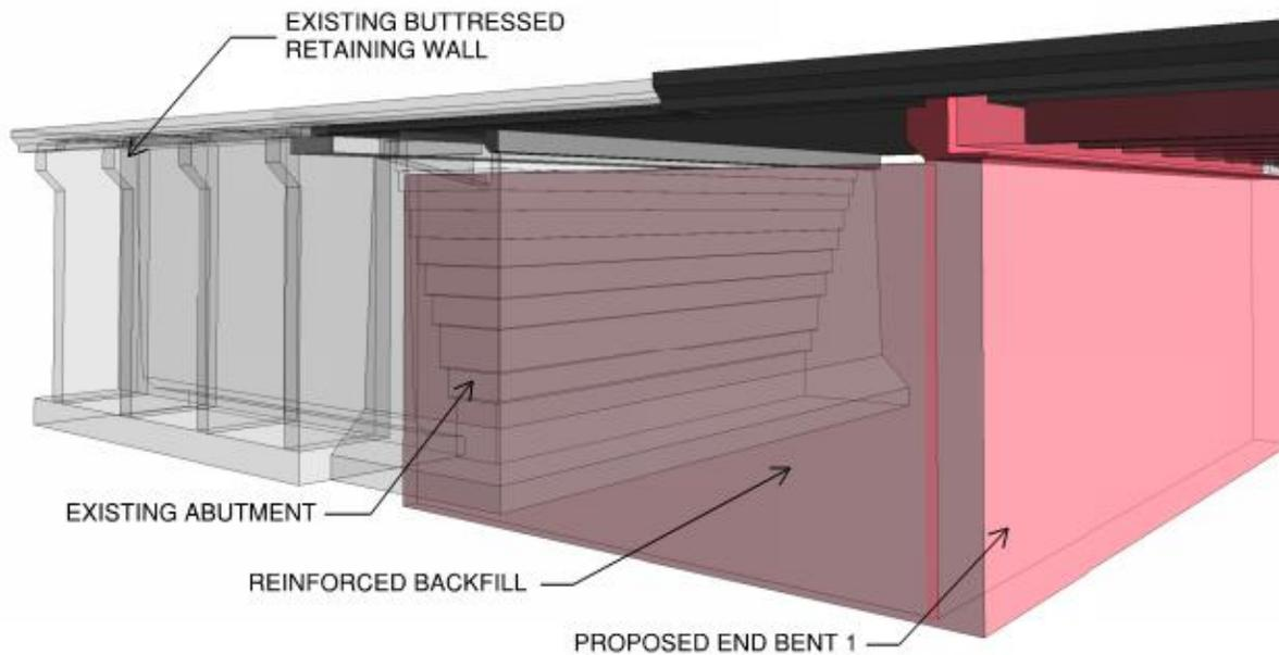
The east approach embankment similarly has both cantilever and buttressed walls past the abutment, however these have already been exposed and backfilled as part of new building construction. It is assumed that these walls would be left in place and the sidewalks would be supported by the embankment.
