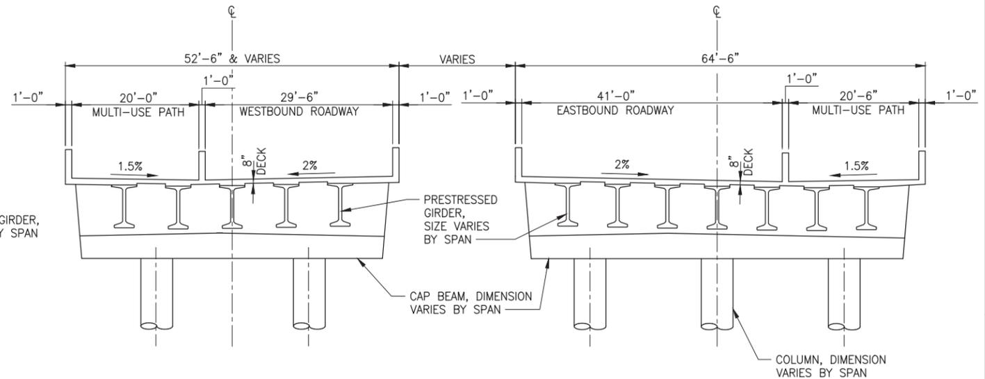
**COUPLER SECTION - PRESTRESSED CONCRETE GIRDER**
