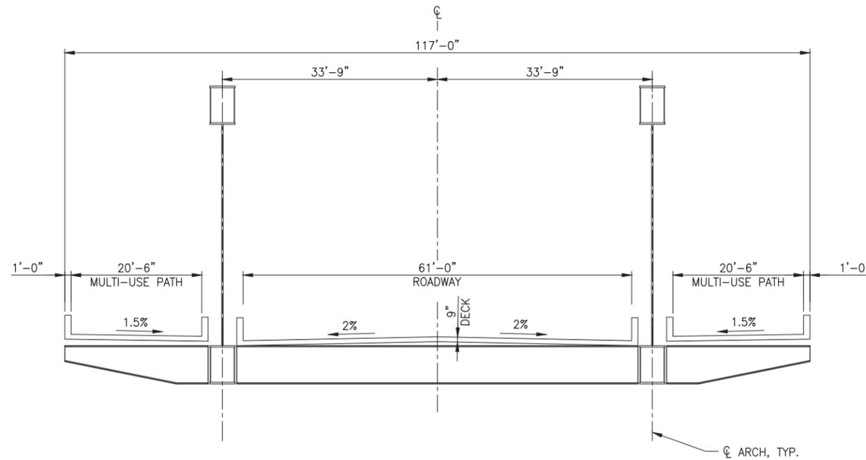
**FULL WIDTH TYPICAL SECTION - STEEL TIED ARCH**
