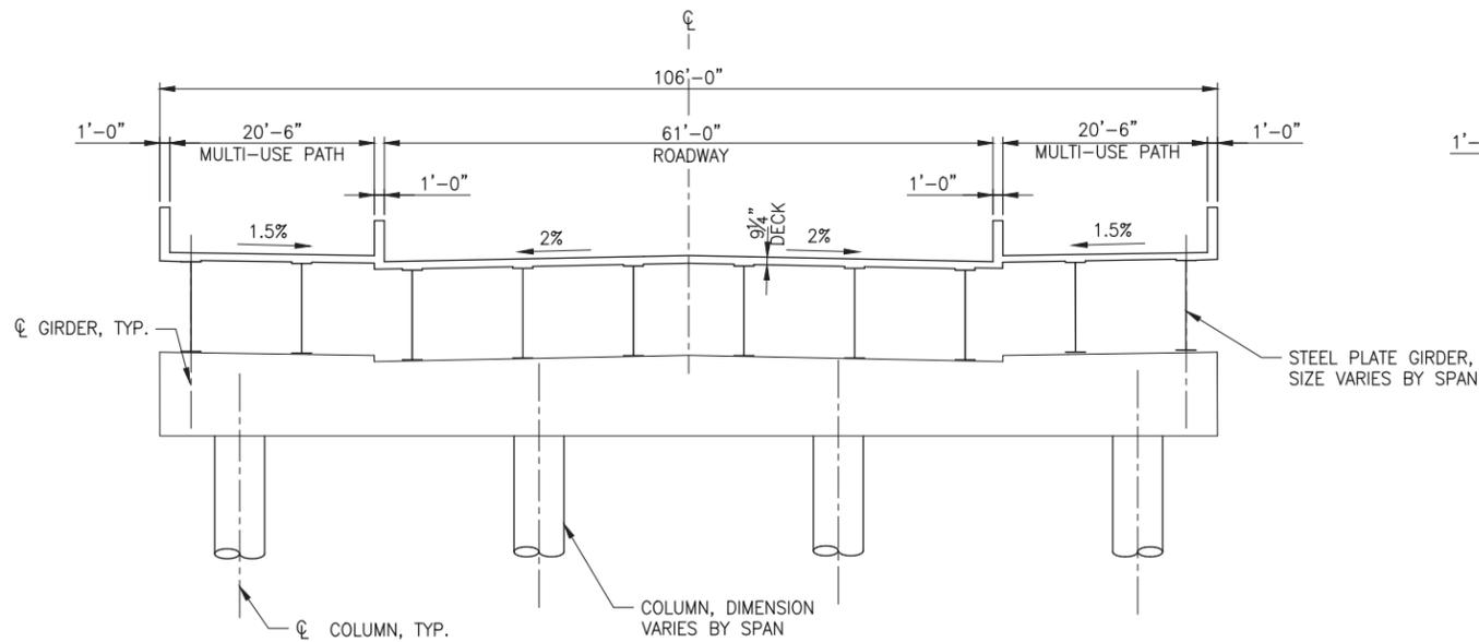
**FULL WIDTH TYPICAL SECTION - STEEL PLATE GIRDER**
