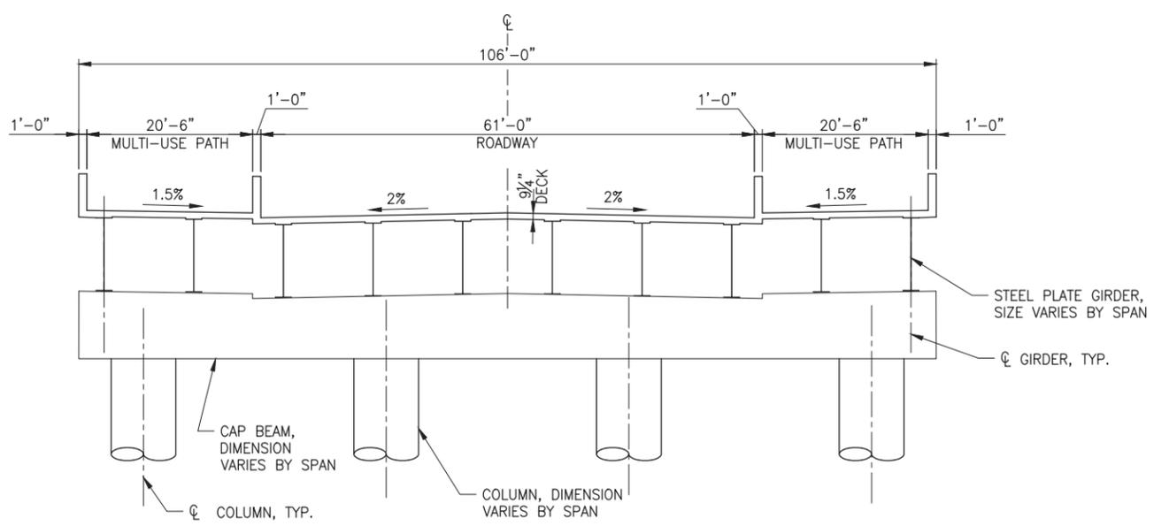
**FULL WIDTH TYPICAL SECTION - STEEL PLATE GIRDER**
