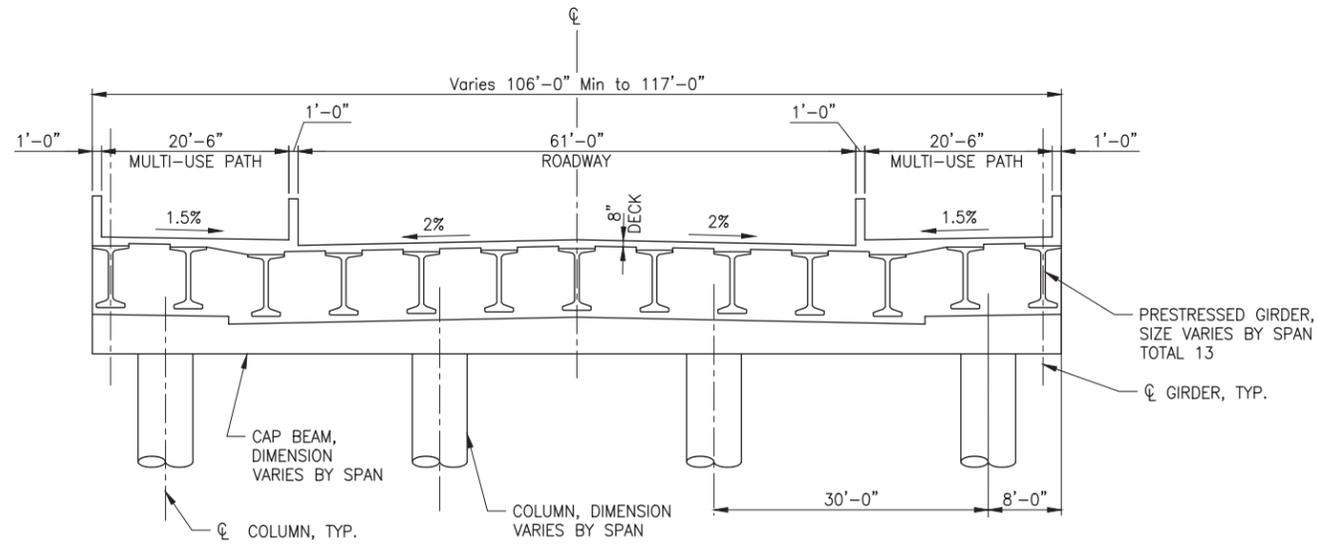
**FULL WIDTH TYPICAL SECTION - PRESTRESSED CONCRETE GIRDER**
