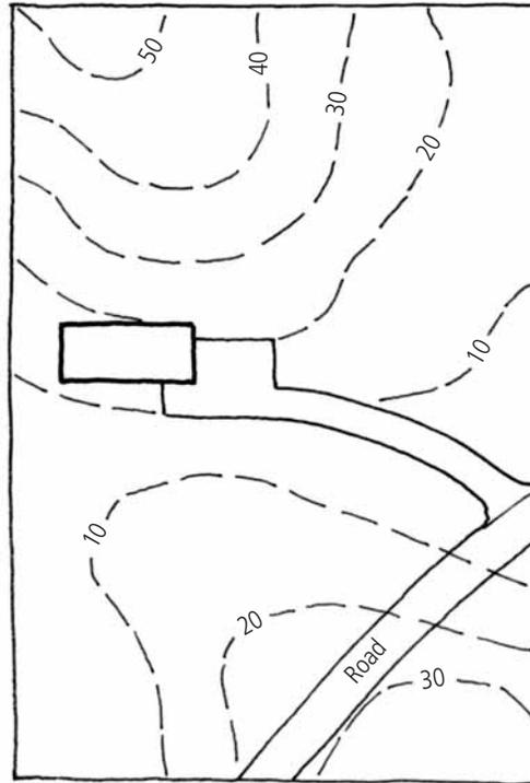
The structure and access drive are aligned with the slope to avoid excessive grading.
