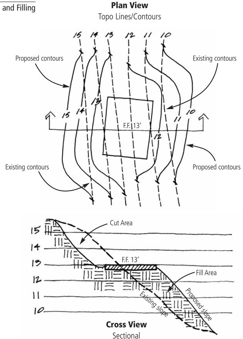
Areas of addition or fill include areas where the proposed elevations (represented by the numbers on the proposed contour lines) are higher than the existing elevations (numbers on the existing contour lines). Conversely, areas of removal or cut include areas where proposed elevations are lower than the elevation of the existing contour lines. Note: This figure exaggerates vertical slopes for illustration purposes.
