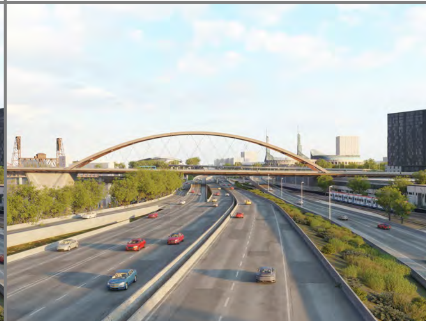
TA2-Braced basket-handle arch
