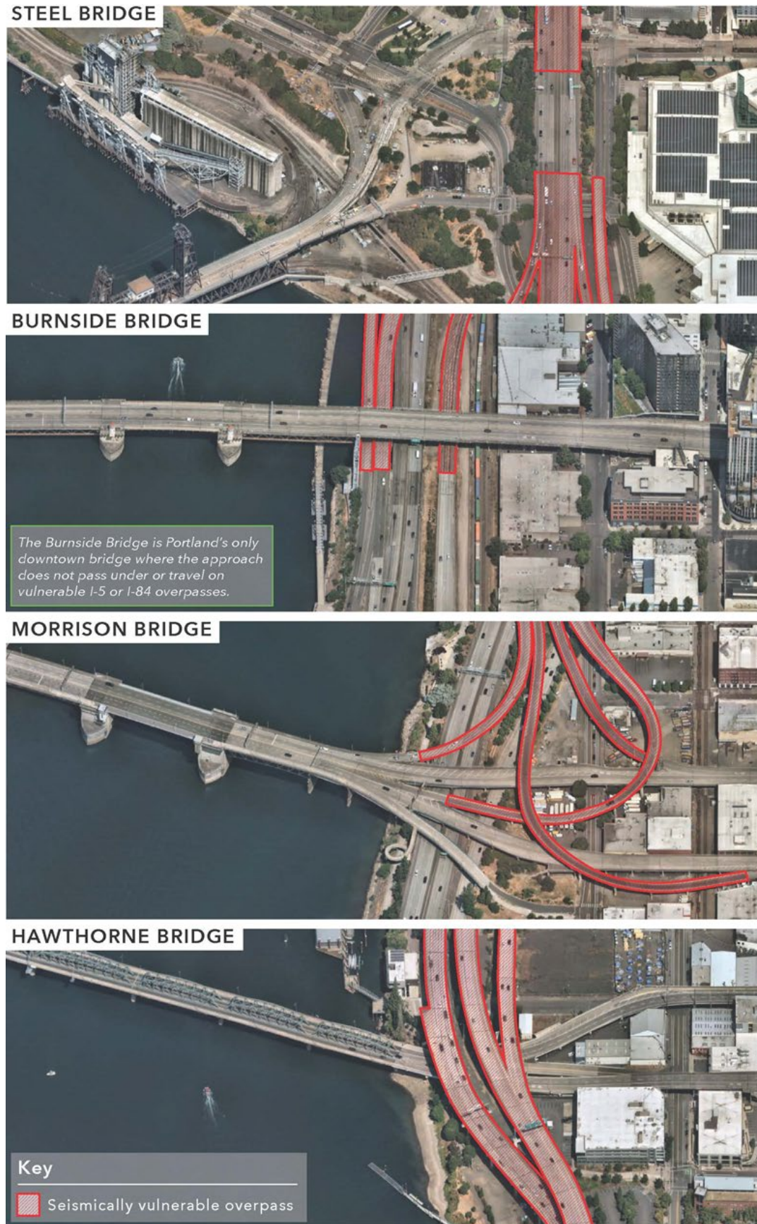
Figure 1.4-3. Seismic Vulnerability of Downtown Bridge Approaches
