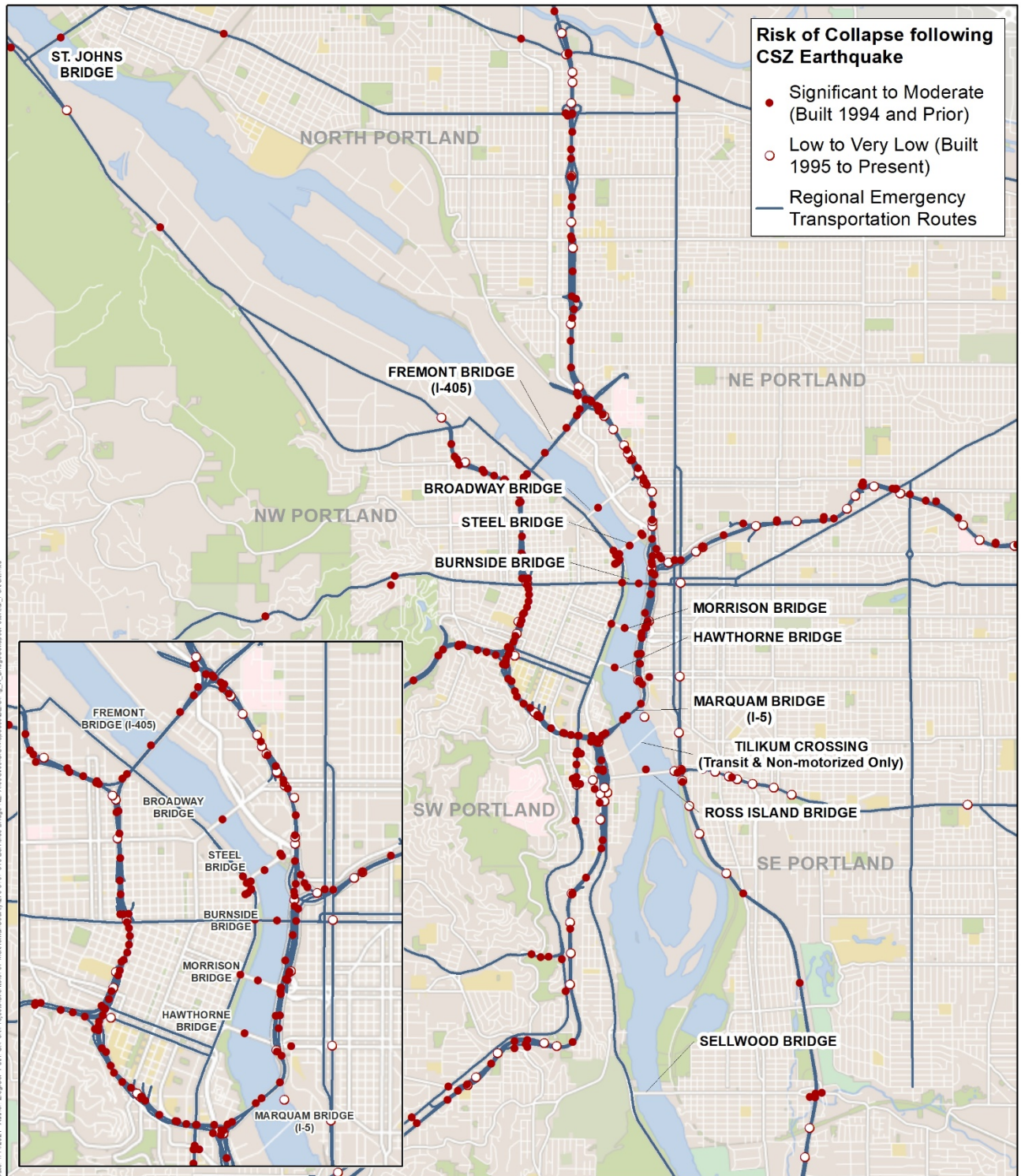
Figure 1.4-2. Risk of Bridge and Overpass Collapse
