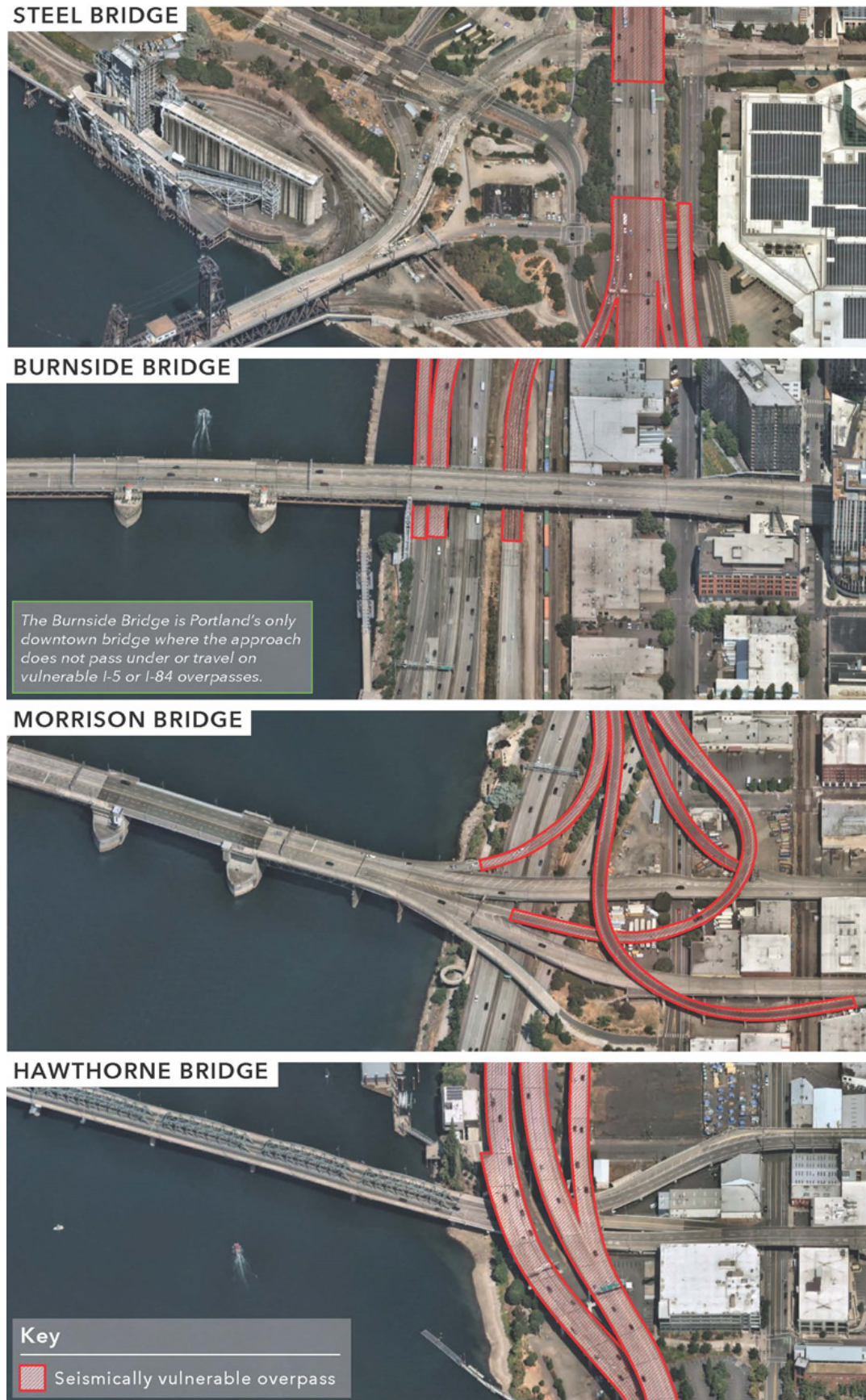
Figure 1.4-3. Seismic Vulnerability of Downtown Bridge Approaches
