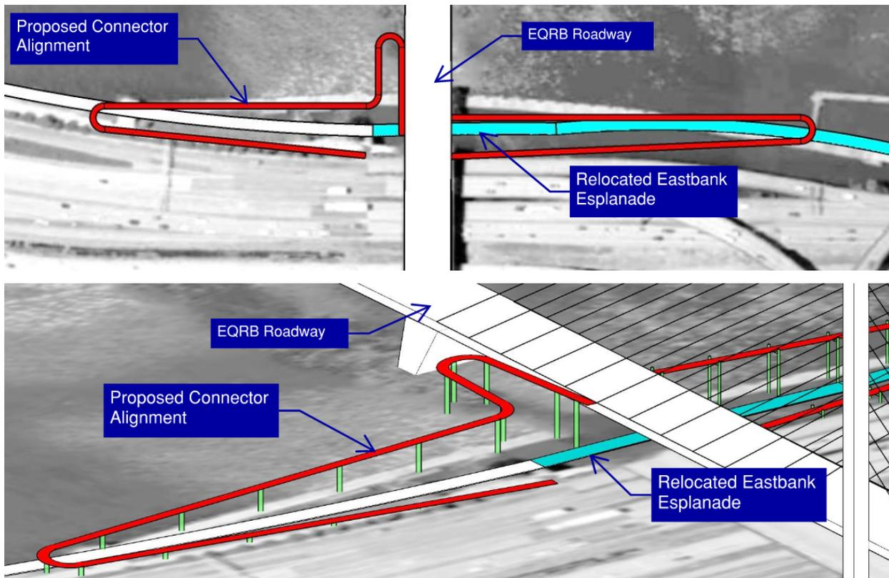
Figure 3: Alignment Concept 1
