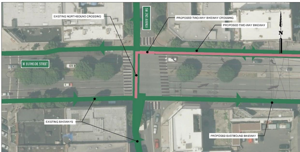
Figure 40. Two-Way Bikeway West Side: Utilize South and East legs to Connect Eastbound Bicyclists to North-Side Two-Way Bikeway
