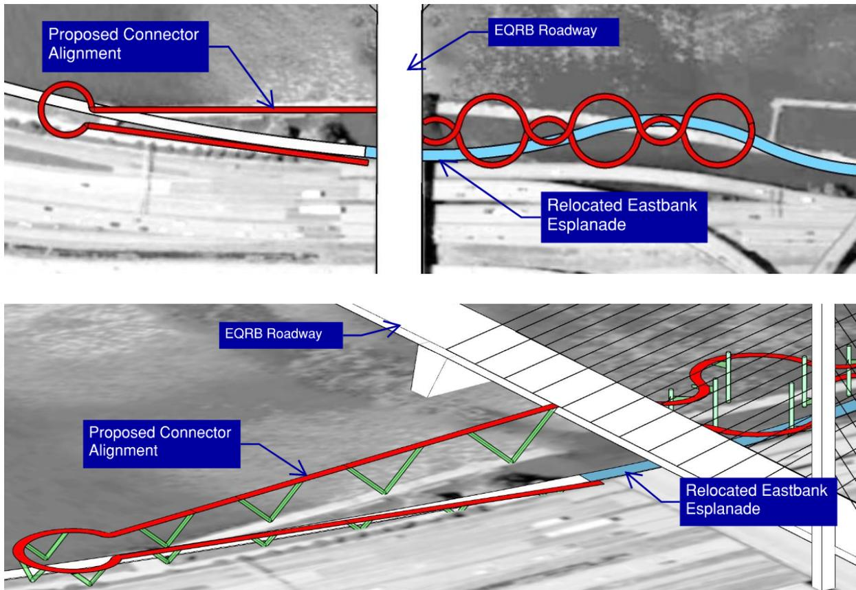
Figure 4: Alignment Concept 2
