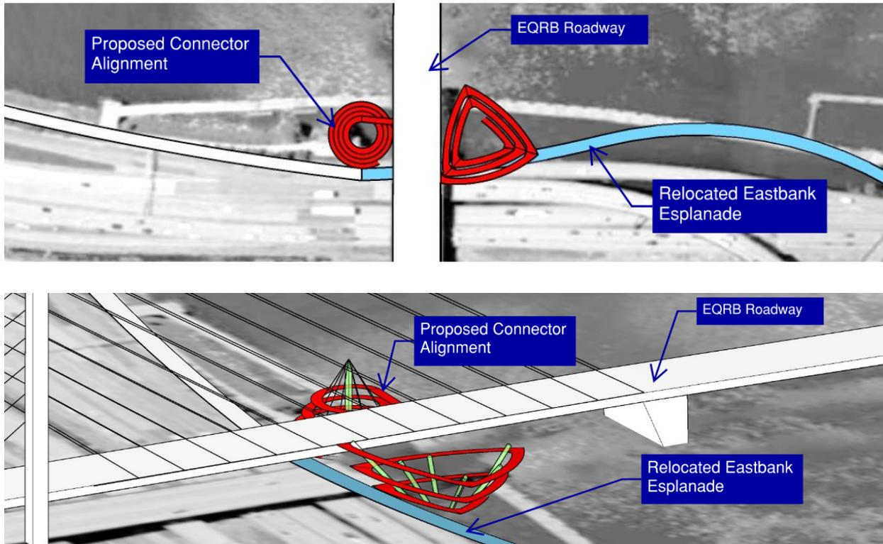
**Figure 5: Alignment Concept 3**
