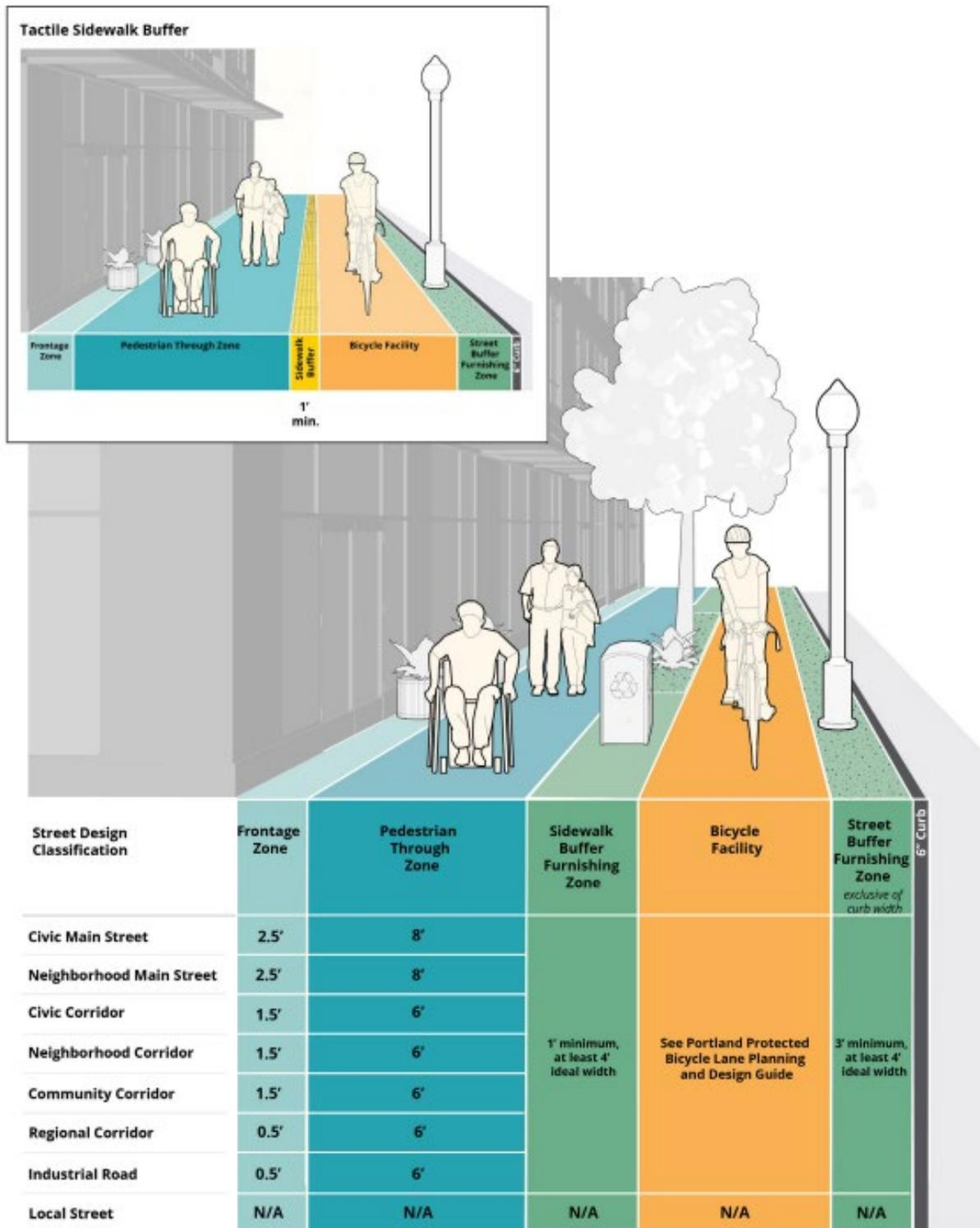
**Figure 16: Portland Protected Bicycle Lane Design Guide Recommended Bike Lane Dimensions**
