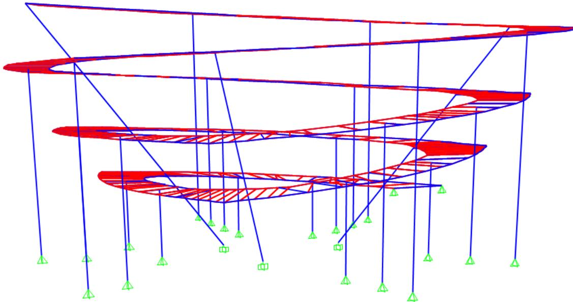
**Figure 10: Rendering of 3D SAP2000 analysis model**
