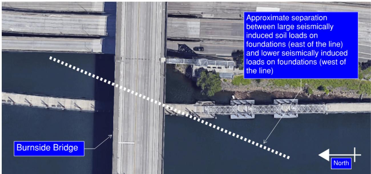
**Figure 2: Plan at Existing Bridge Showing Approximate Location of Liquefiable Soils**
