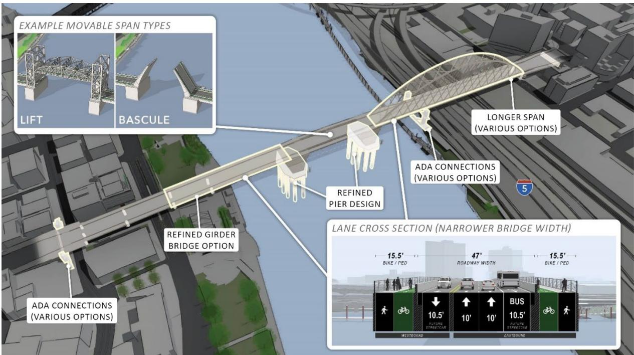
Notes: The Refined Long-span Alternative evaluated in this SDEIS includes both cable-stayed and tied-arch options for the east span. This figure shows only the tied-arch option. The Draft EIS studied, and SDEIS further studies, a bascule option and vertical lift option for the center movable span. The inset shows both options but the main figure shows the bascule option. This figure also shows just one of the lane configuration options considered in the SDEIS.
