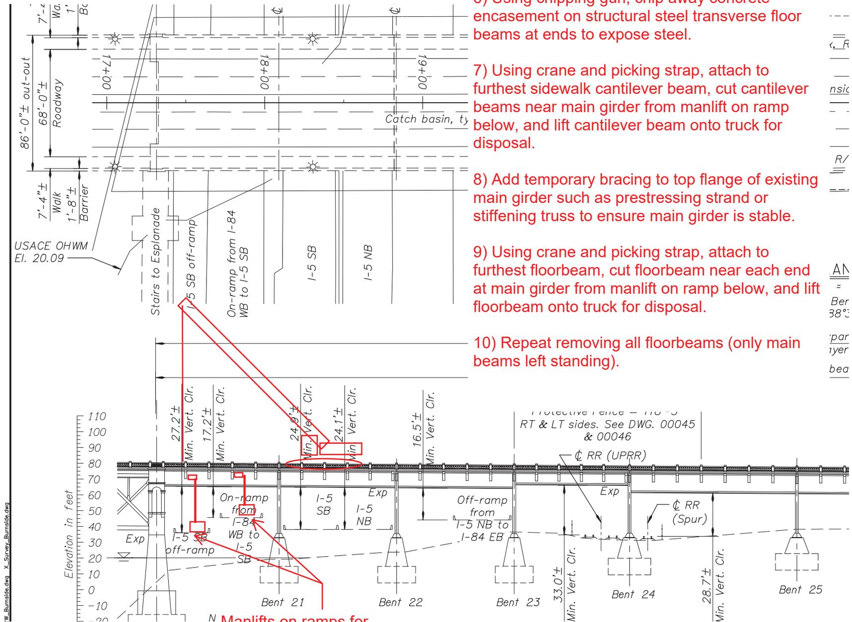
Manlifts on ramps for chipping & burning girders (will be on mainline and I-84 ramp during Span 21 & 22 removal)
