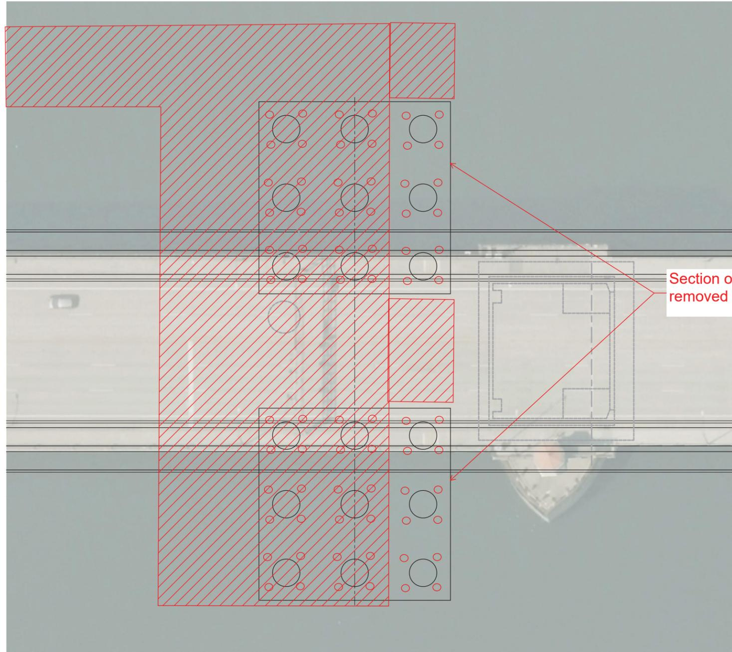
Section of work bridge removed to access shafts
