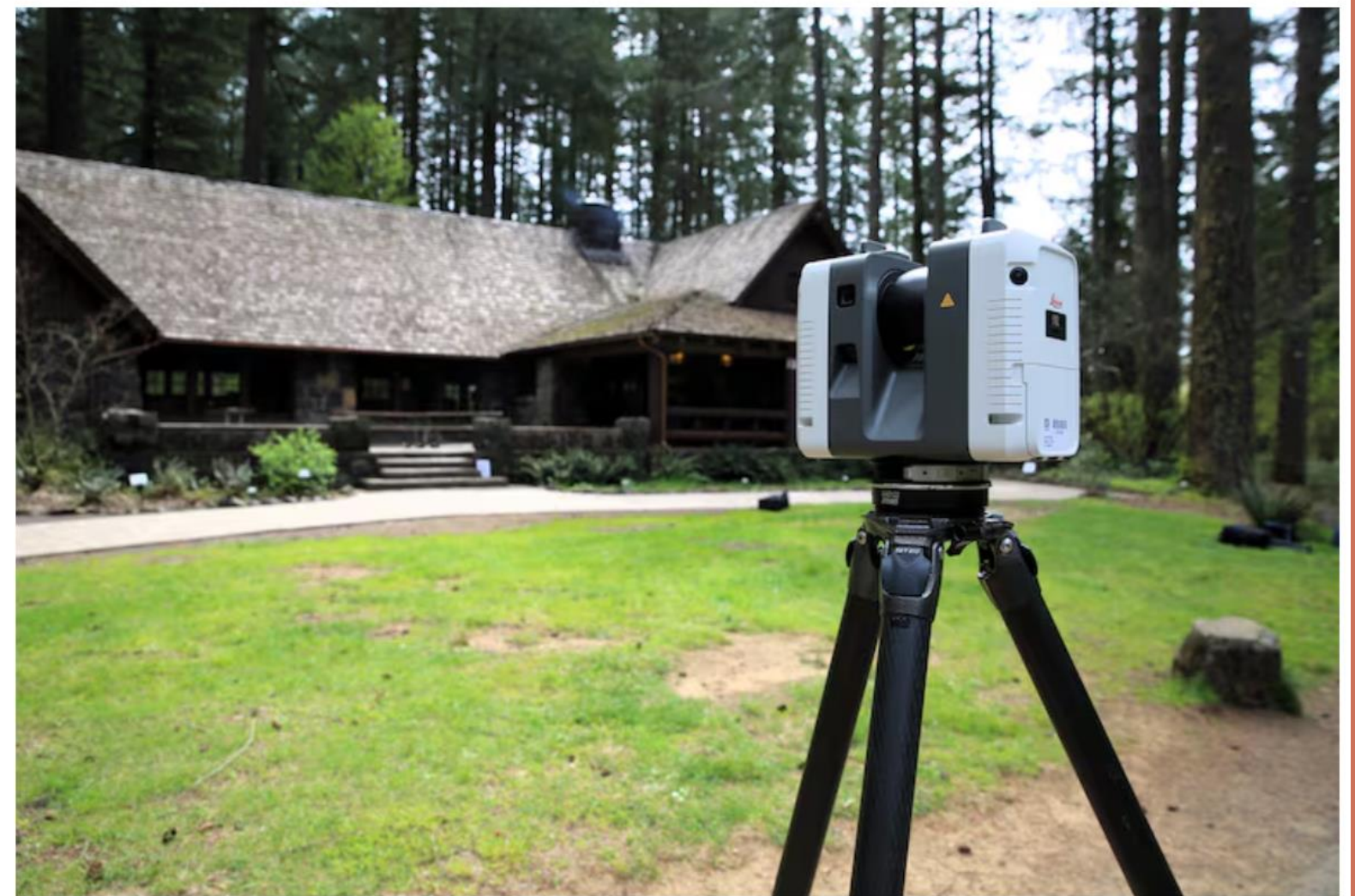
A laser scanner makes a three-dimensional map of Silver Falls Lodge. Kristian Foden-Vencil / OPB
