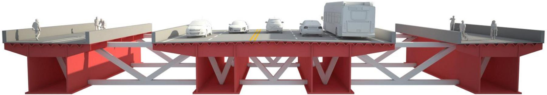
Burnside Bridge Cross Section of Lift Span
