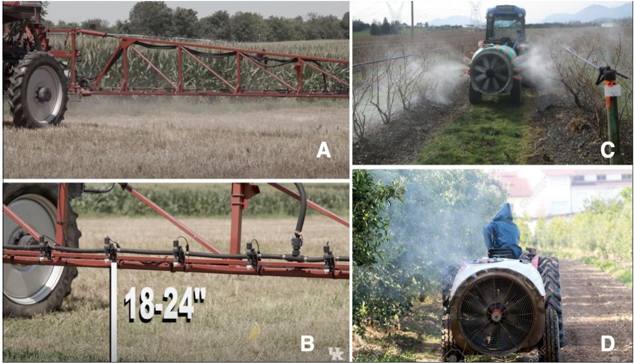
Figure 4. Ground boom sprayer (A,B) used for cereal, grain, and vegetable crops and axial fan airblast sprayer (C,D) used for perennial crops in orchards, vineyards, and nurseries. The boom sprayer simulation for this analysis was run for both low boom (recommended best management practice, B) and high boom (48-50 inches). The airblast sprayer assumed application to a dormant crop canopy (C) and a fully leafed out canopy (D). (Picture credits: A,B from youtube.com/watch?v=4i4a9S0Zpzi ; C from canada.ca/en/health-canada/services/consumer-product-safety/pesticides-pest-management/growers-commercial-users/drift-mitigation/management-pesticide-spray-drift.html ; D from 123rf.com/photo_59922226_air-blast-sprayer-with-a-chemical-insecticide-or-fungicide-in-the-orchard.html )
