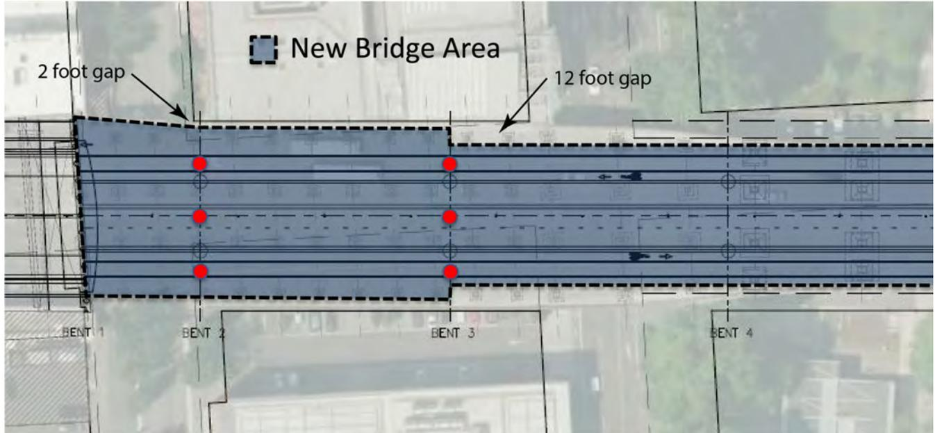
Figure 16: Preliminary engineering drawing showing proposed separation between the new west approach and the south façade of the White Stag Block. Base image courtesy of HDR, Multnomah County, and Earthquake Ready Burnside Bridge Project. Dimensional notations by WillametteCRA (June 2022).
