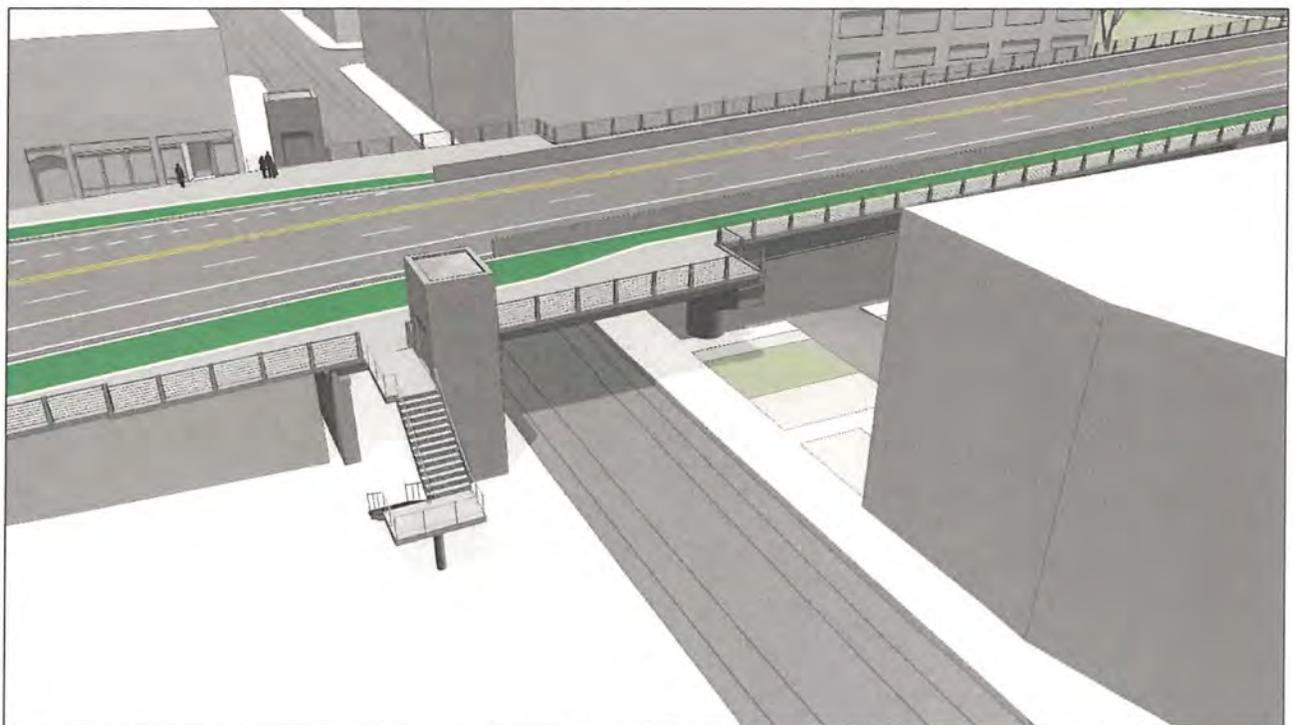
Figure 28: Proposed new pedestrian access at south side of west approach, artist's rendering, aerial view looking northeast (Fat Pencil Studio, 2021). **NOTE: elevators omitted.**
