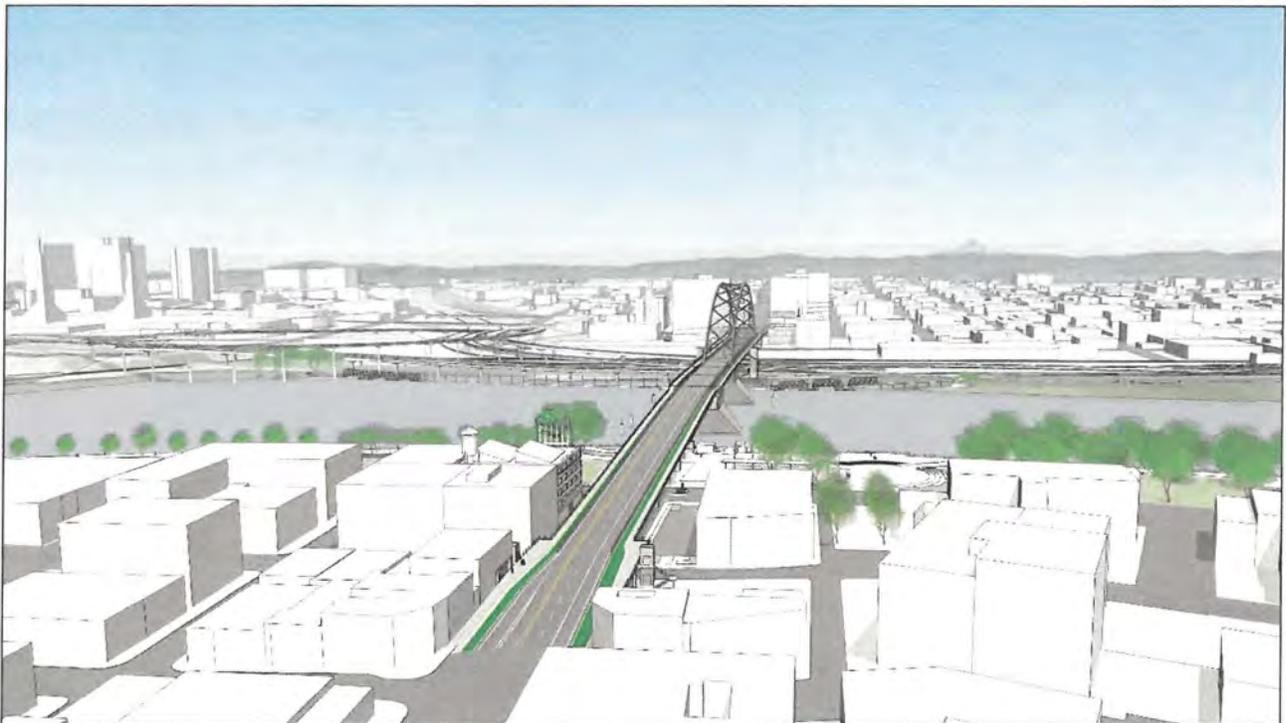
Figure 54: Span Combination 1 (girder west approach, bascule central span, tied arch east approach), artist's rendering, view looking east (Fat Pencil Studio, 2021). **NOTE: elevators omitted.**
