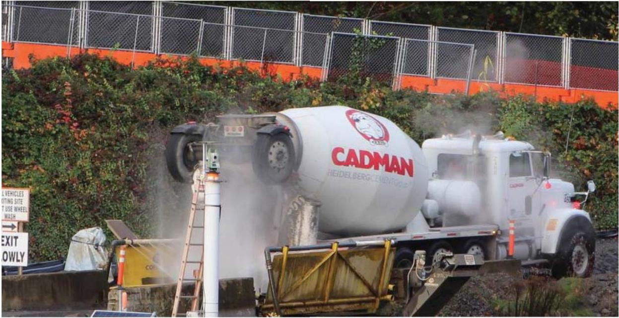
Figure 8. Example of construction truck using a wheel wash before leaving the site.
