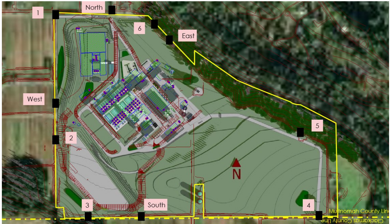
Figure 3. Bull Run Filtration Facility Receiver Locations (indicated in Black Rectangles).
