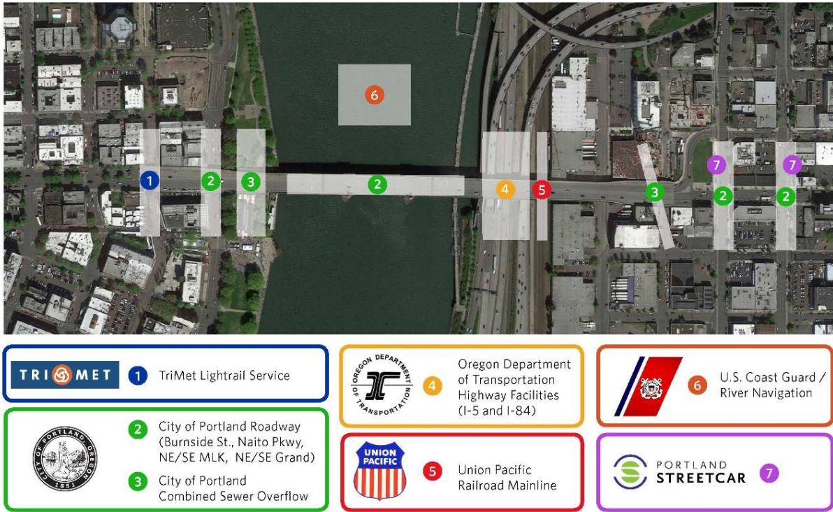
Figure 1-4. Adjacent Major Transportation Facilities and Buildings of Burnside Bridge
