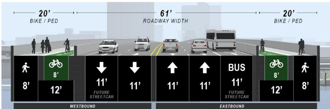
Figure 12. Bridge Cross Section Over River – Refined Long-Span Alternative
