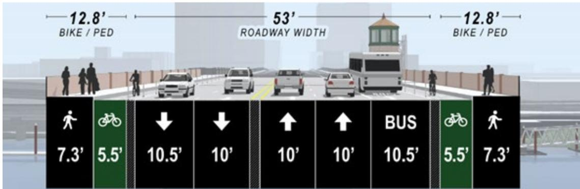
Figure 11. Bridge Cross Section Over River – Draft EIS Long-Span Alternative
