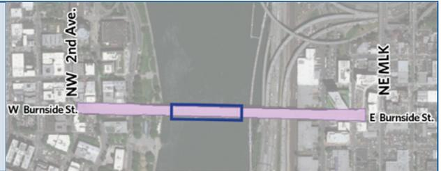
**Northeast Wishbone** – The west landing is full width on the existing Burnside Street alignment; the east landing splits into the existing one-way couplet of NE Couch Street (WB) and Burnside Street (EB).
