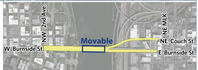
**Southeast Wishbone** – The west landing is full width on the existing Burnside Street alignment; the east landing splits into a one-way couplet with the existing NE Couch Street connection (WB) and the EB lanes diverting to SE Ankeny Street, reconnecting to Burnside Street between SE Grand Avenue and SE 6th Avenue.
