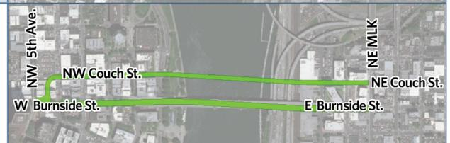
**North Twin Mode Separated** – Vehicular traffic is carried on the existing Burnside Street alignment while bicycle and pedestrian traffic are carried on a separate structure to the north from an extension of NE Couch Street at NE 3rd Avenue to Waterfront Park.
