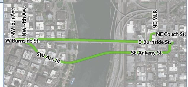
**South Twin Mode Separated** – Vehicular traffic is carried on the existing Burnside Street alignment while bicycle and pedestrian traffic are carried on a separate structure to the south from Waterfront Park to SE Ankeny Street.
