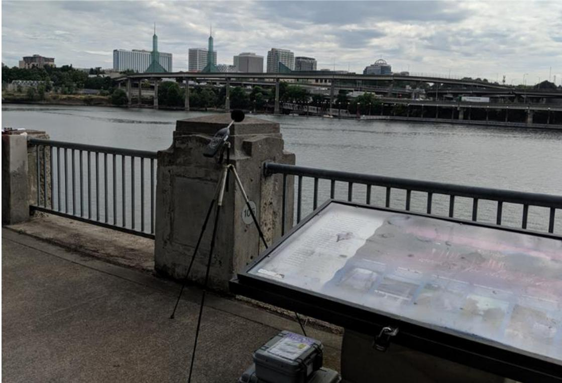
**Photo 2. Site 1: Tripod Mounted Sound Level Meter Tom McCall Waterfront Park North of Burnside Bridge Facing Northeast**
