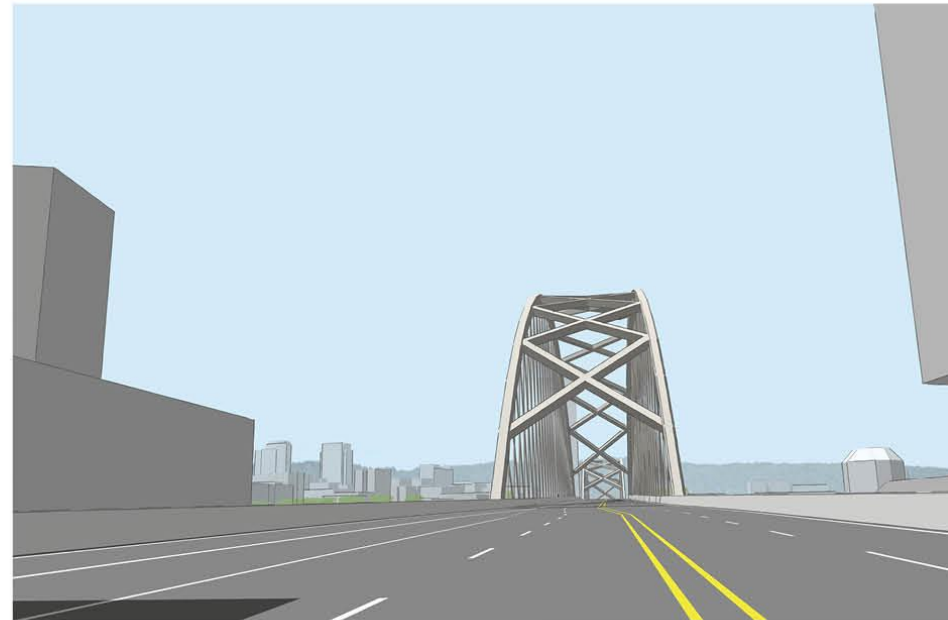
Long-span Alternative / Tied-arch / Bascule
