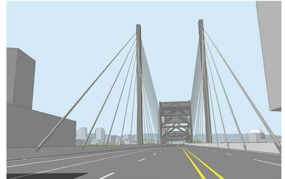
Long-span Alternative / Cable-stayed / Lift
