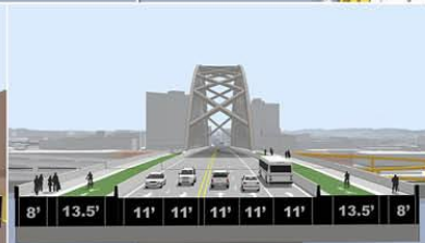
LANE CONFIGURATION AT MID-SPAN
