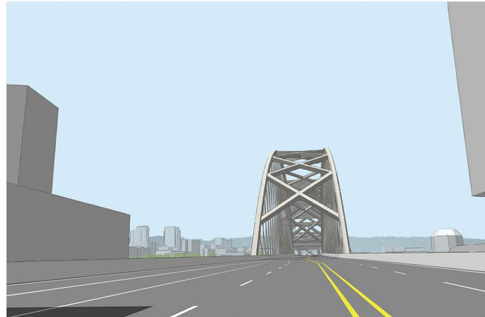
Long-span Alternative / Tied-arch / Lift
