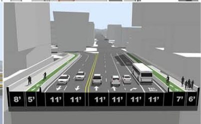
LANE CONFIGURATION AT EAST APPROACH
