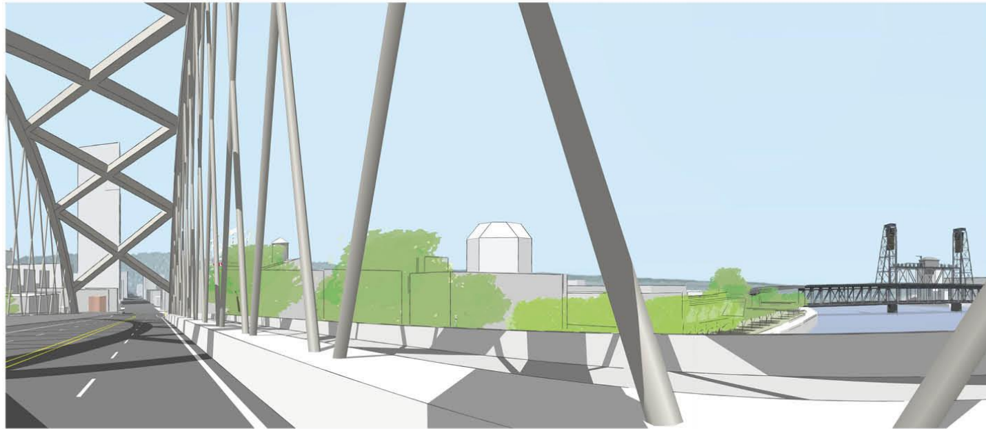
Long-span Alternative / Tied-arch / Bascule
