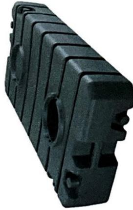
Satellite | Five Peaks 250-gallon holding tank is fitted with six recessed 3" Fernco-style couplings, one 10" manway installed, and a second location where you can install another 10" manway. The deep channels in the tank add strength and rigidity, allowing multiple tanks to be stacked on top of each other without warping.
