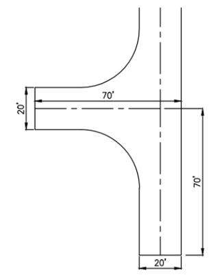
**HAMMERHEAD TYP. GEOMETRY**
