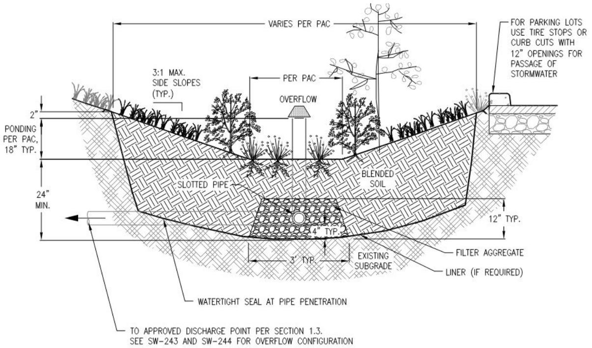
**Figure 3: Bureau of Environmental Service standard detail SW- 231, "Planter – Unlined"**
