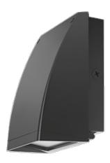
37, 57 and 62 Watt SLIM Wall packs are designed to cover the footprint of most traditional wall packs. They are suitable for mounting heights from 20' to 30', and replace HID Wattages from 200W MH to 320W MH. These ultra-high efficiency fixtures are available in cutoff or full cutoff models.
