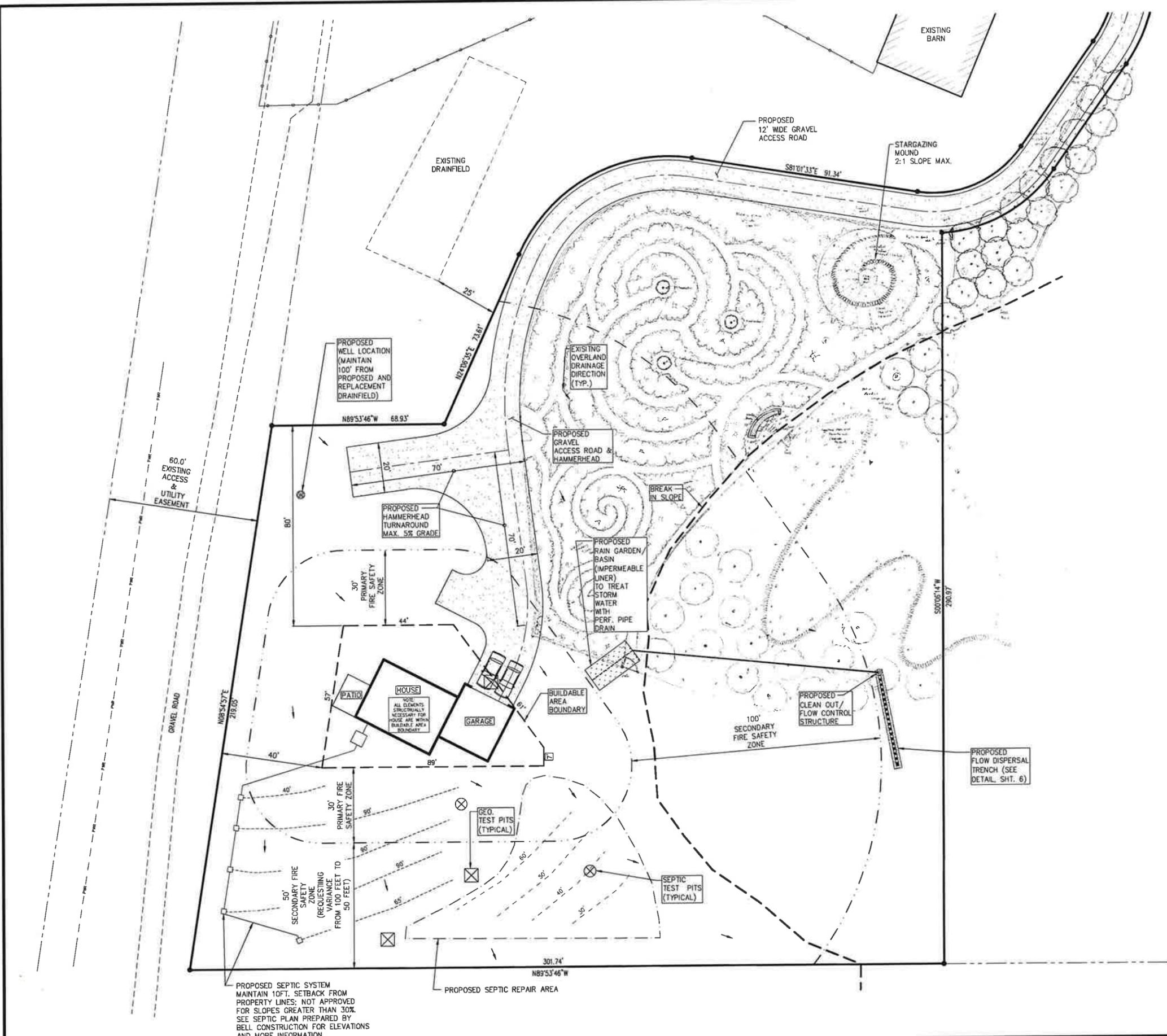
PROPOSED SEPTIC SYSTEM MAINTAIN 10FT. SETBACK FROM PROPERTY LINES; NOT APPROVED FOR SLOPES GREATER THAN 30%. SEE SEPTIC PLAN PREPARED BY BELL CONSTRUCTION FOR ELEVATIONS AND MORE INFORMATION.
