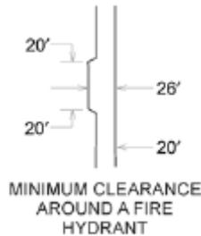
**NO PARKING SIGNS:** Where fire apparatus roadways are not of sufficient width to accommodate parked vehicles and 20 feet of unobstructed driving surface, “No Parking” signs shall be installed on one or both sides of the roadway and in turnarounds as needed. Roads 26 feet wide or less shall be posted on both sides as a fire lane. Roads more than 26 feet wide to 32 feet wide shall be posted on one side as a fire lane.
