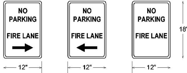
**PAINTED CURBS:** Where required, fire apparatus access roadway curbs shall be painted red (or as approved) and marked "NO PARKING FIRE LANE" at 25' intervals. Lettering shall have a stroke of not less than one inch wide by six inches high. Lettering shall be white on red background (or as approved). (OFC 503.3)
