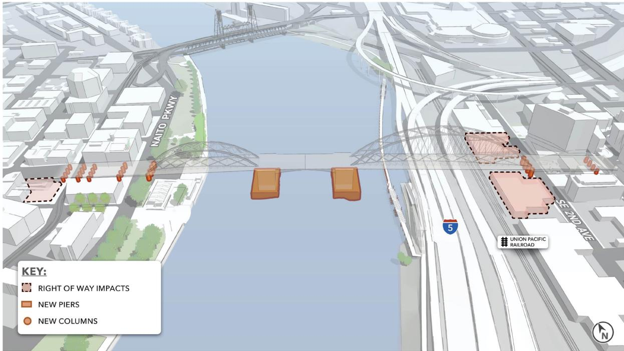
**Figure 10. Long-Span Alternative: Bascule Lift Option and Tied-Arch Configuration**
