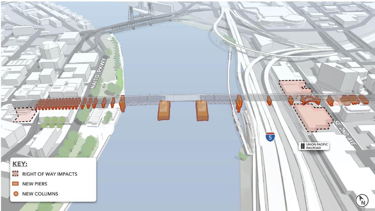
Figure 3. Enhanced Seismic Retrofit: Pier and Bent Locations – Plan View
