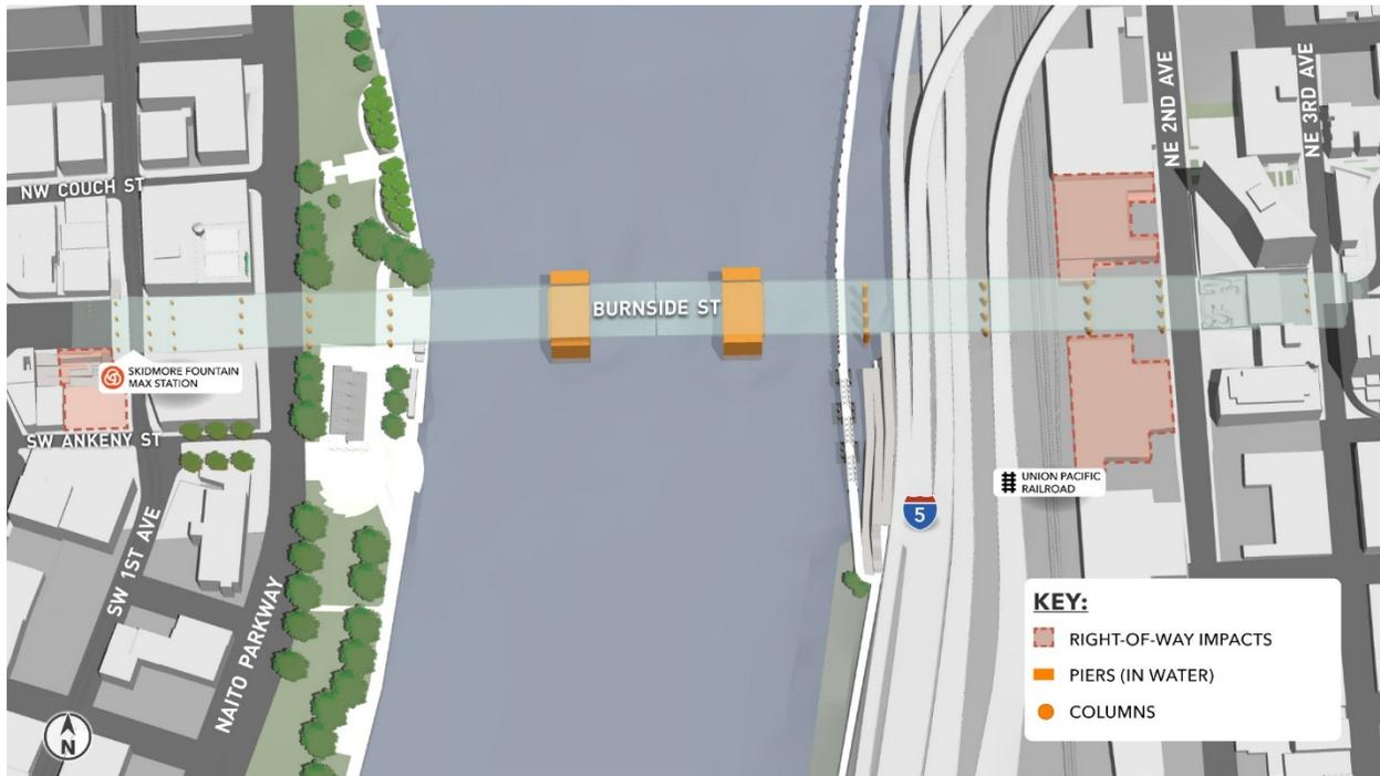
Figure 6. Short-Span Alternative: Configurations and Bent Locations
