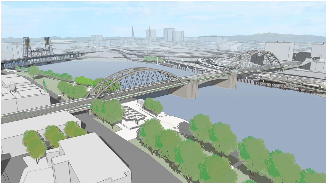
Figure 11. Long-Span Alternative: Vertical Lift Option and Tied-Arch Configuration
