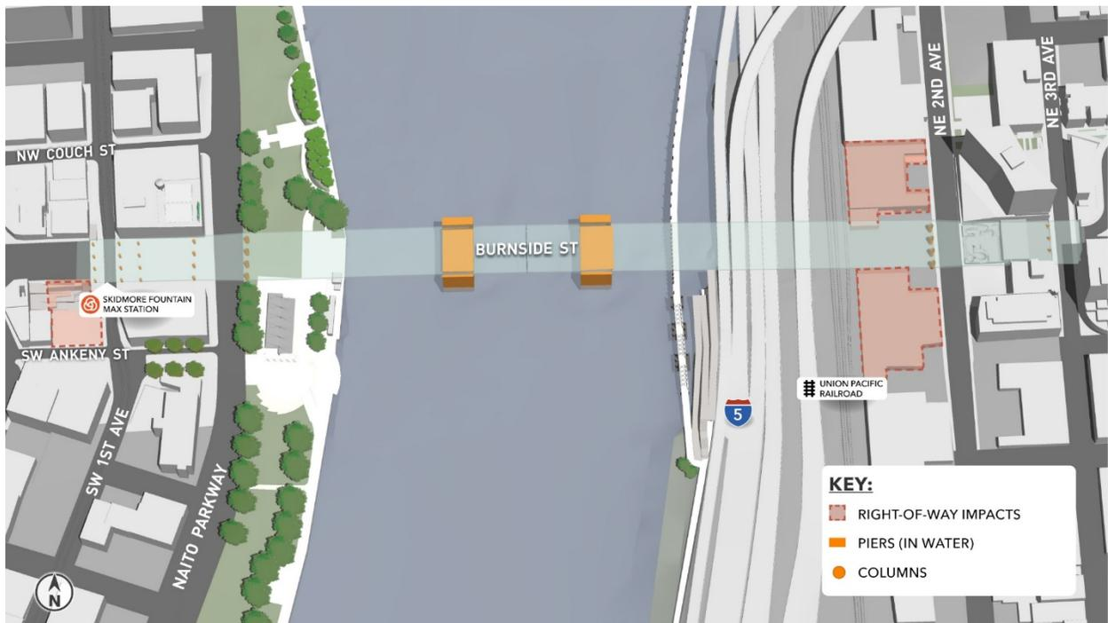
**Figure 9. Long-Span Alternative: Configurations and Bent Locations (Tied-Arch Configuration with Generic Movable Span Shown)**
