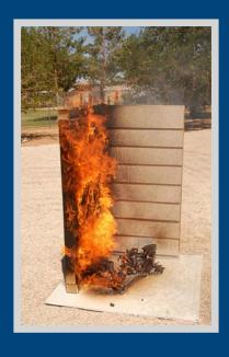
This test photo shows how flames from burning combustible siding can spread upward and expose windows and eaves to flames. The siding that isn't burning is a noncombustible product. Even though it had the same initial fire exposure, the siding did not ignite.
