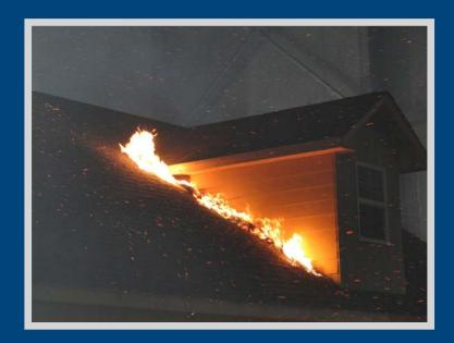
This test photo shows how burning debris at the intersection of the roof and walls exposes the wall to direct contact with flames once the debris is ignited by wind-blown embers.
