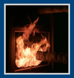
This test photo illustrates how flames can break the glass in a window and penetrate into the interior of a home. Having a dual-pane, tempered glass window offers the best protection because tempered glass does a much better job resisting breakage and even if the outer-pane of glass breaks, the inner pane may remain intact. Keep all windows closed during wildfires – the most vulnerable window during a wildfire is one that is left open.
