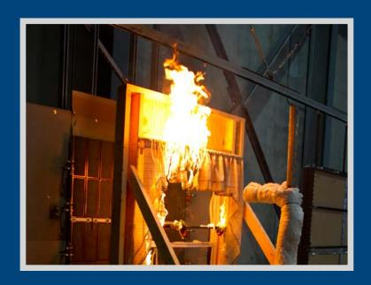
IBHS conducted a test to see whether cotton curtains ignited when exposed to radiant heat that might threaten a window during a wildfire. This test photo shows the curtain burning. However, the curtain only ignited after the glass broke and fell out of the window. This reinforces the advantage of using dual-pane windows, particularly those with tempered glass in the outside panel for the best wildfire protection.
