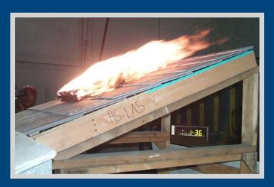
Fire ratings include Class A, B or C. This photo shows testing of a roof covering using a Class A brand, which is the largest of three sizes used in the rating tests. If the burning Class A brand doesn't result in fire penetrating completely through the roof covering and sheathing into what would be the attic space, then the roof covering would earn a Class A fire rating.
